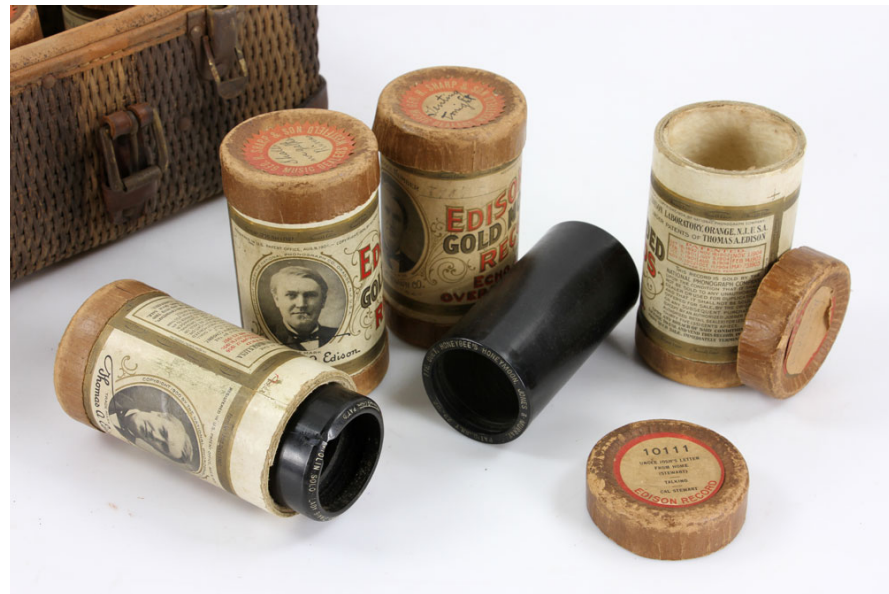
Fig: Wax Cylinders, most popular around 1896–1916 with a capacity of about 2 minutes.
