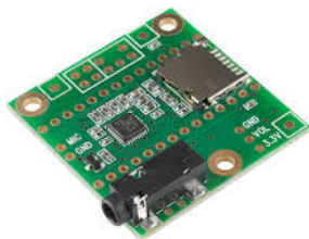
Fig: The Audio Adapter Board for Teensy adds audio capabilities to a Teensy
