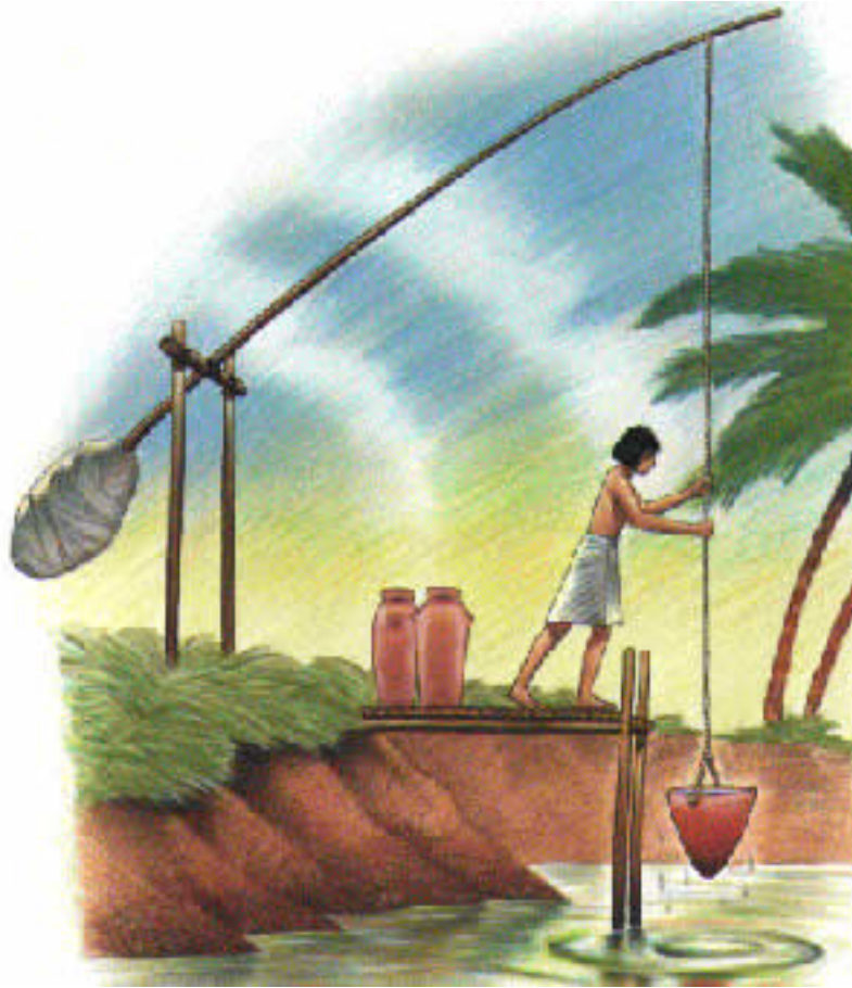
Illustration 1. A shaduf was used to raise water above the level of the Nile.
