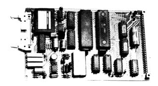
The analog interface offers the Acorn system user laboratory standard facilities for the examination and control of analog signals. It is a  $100\text{mm} \times 160\text{mm}$  Eurocard and connects to the standard Acorn bus using a 64-way indirect connector (DIN 2-row) and employs the following devices:-
