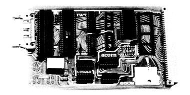
The 6502 CPU is designed for use in the Acorn systems 2,3 and 4 and it plugs onto the standard Acorn 8 or 14 slot backplanes. The 6502 microprocessor is run from a IMHz crystal controlled clock and a TTL device provides address decoding.
