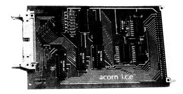
The In-Circuit Emulator (ICE) allows a computer system employing the standard Acorn data bus to connect to a second microprocessor target system by way of its processor chip socket. Once established this connection may be used to test hardware and to evaluate software in the target system. The ICE is extremely useful in the development of new microprocessor products and in the test and repair of existing equipment.
