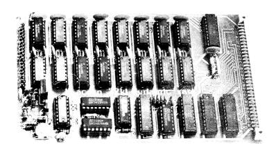
This Eurocard provides 32768 bytes of Random Access Memory for a computer system using the Acorn standard data bus. Such systems include any Acorn or Control Universal (CUBIT range) computer, or a computer using the Acorn bus as an expansion bus, as achieved with the Rockwell AIM 65 using the CUBIT extension system.
