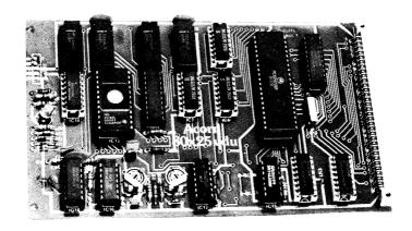
The VDU interface is a  $100 \times 160 \text{nm}$  Eurocard which connects via a 64-way plug and socket to the standard Acorn computer bus. It produces a 1 volt composite signal which drives the 75 ohm input on a monitor.
