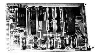
The Visual Display Unit Controller board connects to the standard Acorn bus, as used by Acorn Eurocard products and CUBIT computers and bus extensions. It provides a TV display for all such systems with 1k of RAM memory mapped on the host computer data bus. Text and Teletext graphics are transparently written onto the screen by the CPU.
