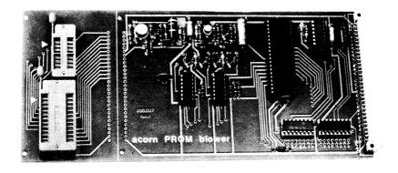
This board conects to the standard Acorn bus and may be used to program bipolar PROMs of the 74S571 type and PROMs types 2758, 2516, 2716 and 2532 ie. 5v only 1K, 2K and 4K byte devices.
