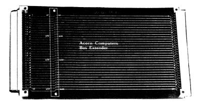
The Acorn Bus Extender is a Eurocard (100mm x 160mm) which plugs into any backplane plug using the DIN 64 way two row a/b socket. This brings the 64 connections to the front of the Eurocard rack where a socket projects out. Any other Eurocard can then be plugged into the extender card, leaving the Eurocard clear of the rack for easy access, allowing it to be serviced or developed while operating in the system.
