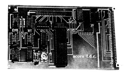
This Eurocard (100 x 160 mm) connects to the standard Acorn bus and provides an interface to one or two drives. It is capable of controlling four drive surfaces on two double sided drives. Single or double track density drives may be used. A 34-way flat ribbon connects to the drives after the Shugart interface standard. The intelligent device used is the Intel 8271. A number of disk operating systems are available for use in various systems.
