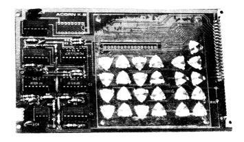
The upper Eurocard of the system 1 is available without keypad and display when it performs as a cassette interface card in system 2. It may also be added to systems 3 and 4 if desired. The Computer Users Tape Standard (CUTS) frequency-modulates data on to a standard audio cassette recorder with two tone system in which 2.4KHz represents a logic 1 and 1.2KHz a logic 0.
