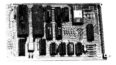
This Eurocard ( $100 \times 160 \text{ mm}$ ) is a plug—in replacement for the 6502 CPU card to upgrade Acorn Systems 3 and 4 to use the advanced facilities of Motorola's 6809 8-bit processor and is ideally suited to run high level languages such as Pascal. The Acorn 6809 is provided with an operating system in 2K which handles the Acorn VDU, ASCII encoded keyboard and printer; it is readily expanded and very user friendly.
