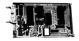
This board connects to the standard Acorn bus and provides interfaces via the three integrated circuits listed below.
