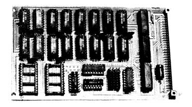
This Eurocard offers 8k of static RAM plus two sockets which each can accept a 4k ROM or EPROM. The 8k RAM bank and the 8k ROM bank can be independently located in memory to commence in 8k intervals throughout the memory may. eg. each may commence at hex 0, 2000, 4000 etc, though to FOOO.
