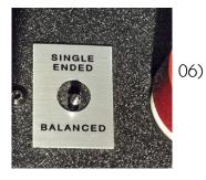
Set the top switch to Balanced (for use with balanced sources on XLR connector) or Single-ended (via RCA connector) as desired.
