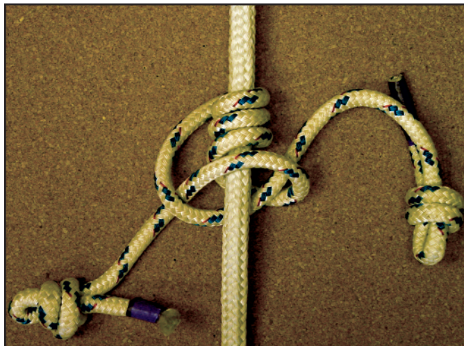
Figure 4. Tying the Martin: The split-tail makes four counterclockwise turns up the climbing line. The top leg is dropped in front of the bottom leg, behind the climbing line and up through the bottom turn.
