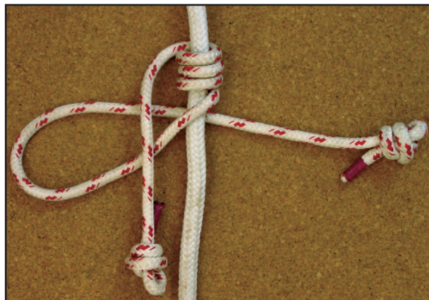
Figure 2. . . . The bight is twisted from bottom to top, away from the climbing line, . . .
