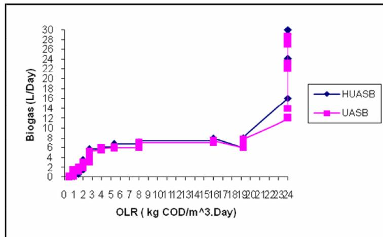
Fig 5: Observed biogas production for the fed OLR
