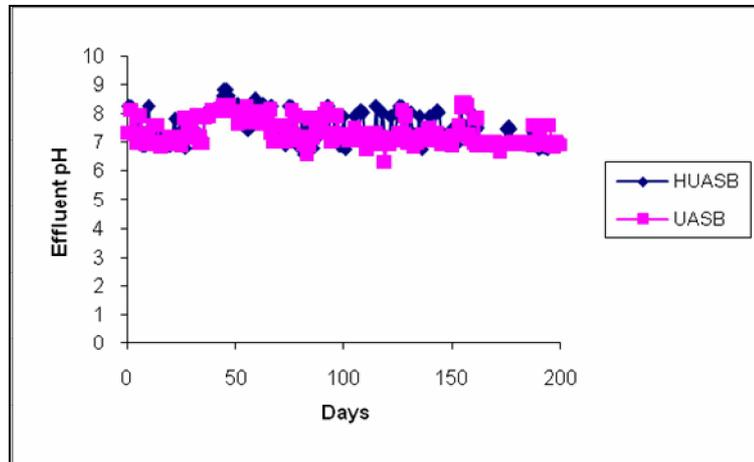
**Fig 7: Variation of effluent pH observed during the study**
