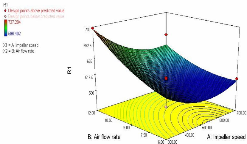
Fig 2 - Response surface plot showing the effect of impeller speed and air flow rate and their interactive effect on the volumetric mass transfer coefficient for 2 L sodium sulphite oxidation method
