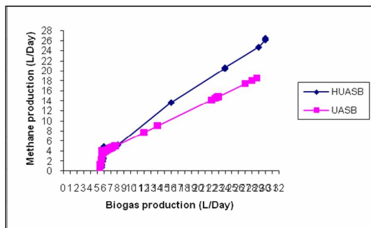
Fig 6: Biogas Vs Methane production observed during the study
