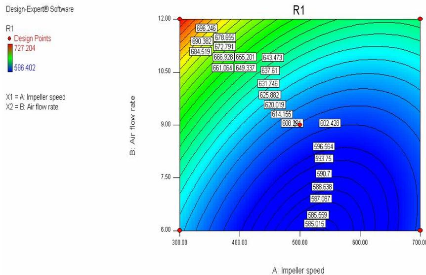
**Fig 1 - Isoresponse contour plots showing the effect of impeller speed and air flow rate and their interactive effect on the volumetric mass transfer coefficient for 2 L sodium sulphite oxidation method.**
