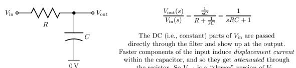
$$\frac{V_{\text{out}}(s)}{V_{\text{in}}(s)} = \frac{\frac{1}{sC}}{R + \frac{1}{sC}} = \frac{1}{sRC + 1}$$
