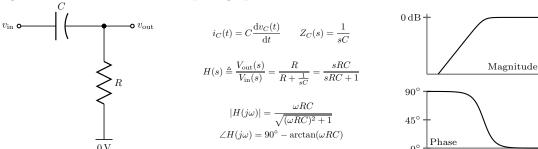
As before, the magnitude response of the filter can be explained by likening the capacitor to an open circuit at low frequencies (i.e., impedance magnitude  $|1/(j\omega C)|$  is near infinity for  $\omega \approx 0$ ) and a short circuit at high frequencies  $(|1/(j\omega C)| \approx 0$  when  $\omega \approx \infty$ ). That is,
