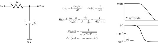
The magnitude response of the filter can be explained by likening the capacitor to an open circuit at low frequencies (i.e., impedance magnitude  $|1/(j\omega C)|$  is near infinity for  $\omega \approx 0$ ) and a short circuit at high frequencies  $(|1/(j\omega C)| \approx 0$  when  $\omega \approx \infty$ ). That is,
