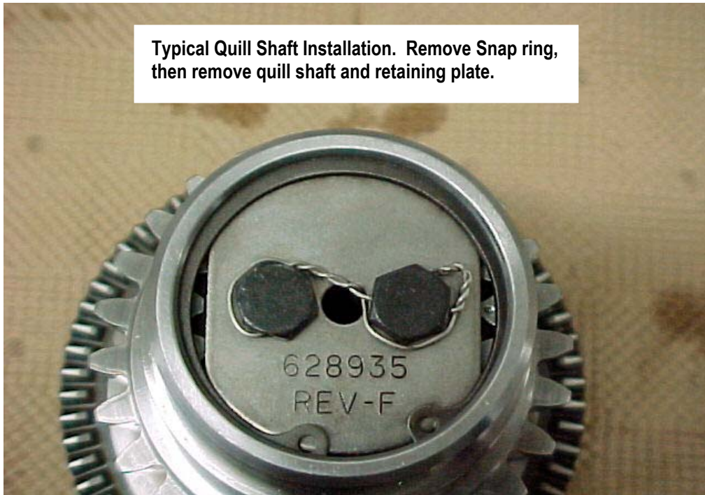
FIGURE 3. QUILL SHAFT INSTALLATION
