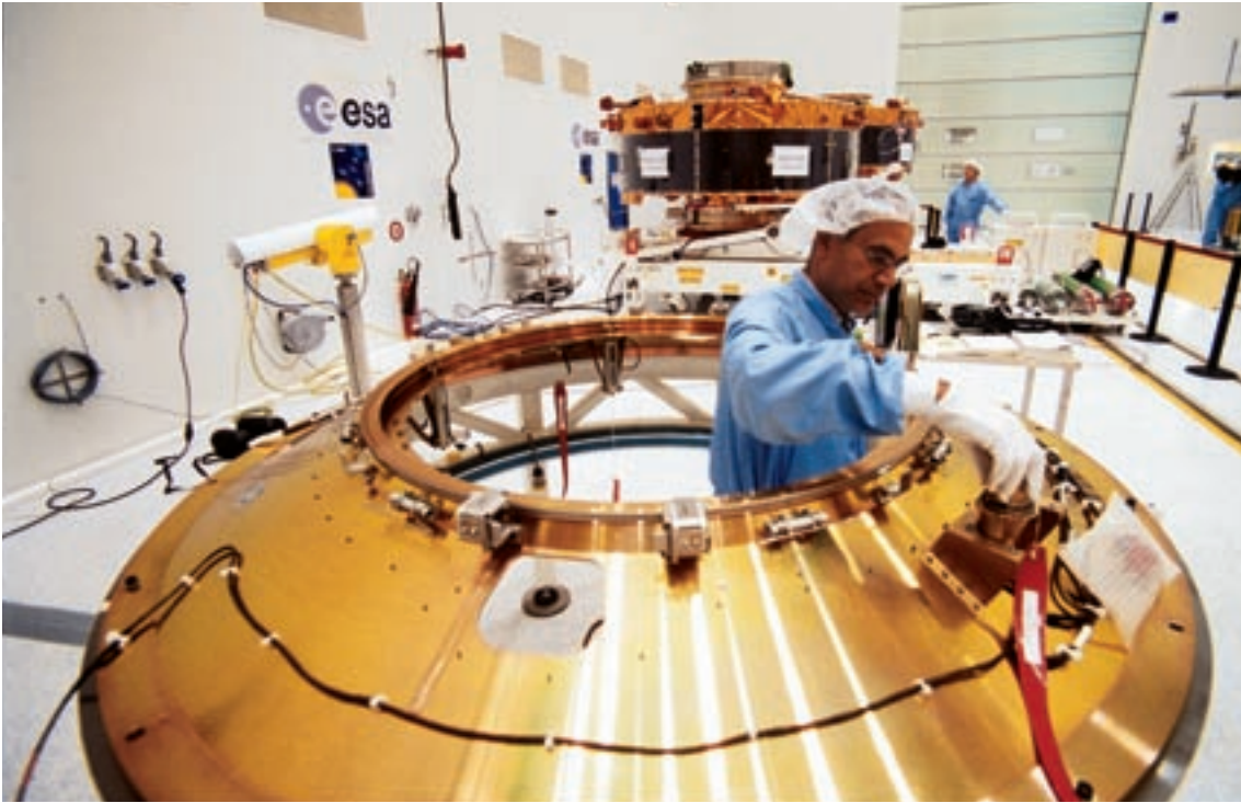
Figure A 2 - 1: Adapter 1194-SF on Its Integration Support Inside the Upper Composite Integration Facility
