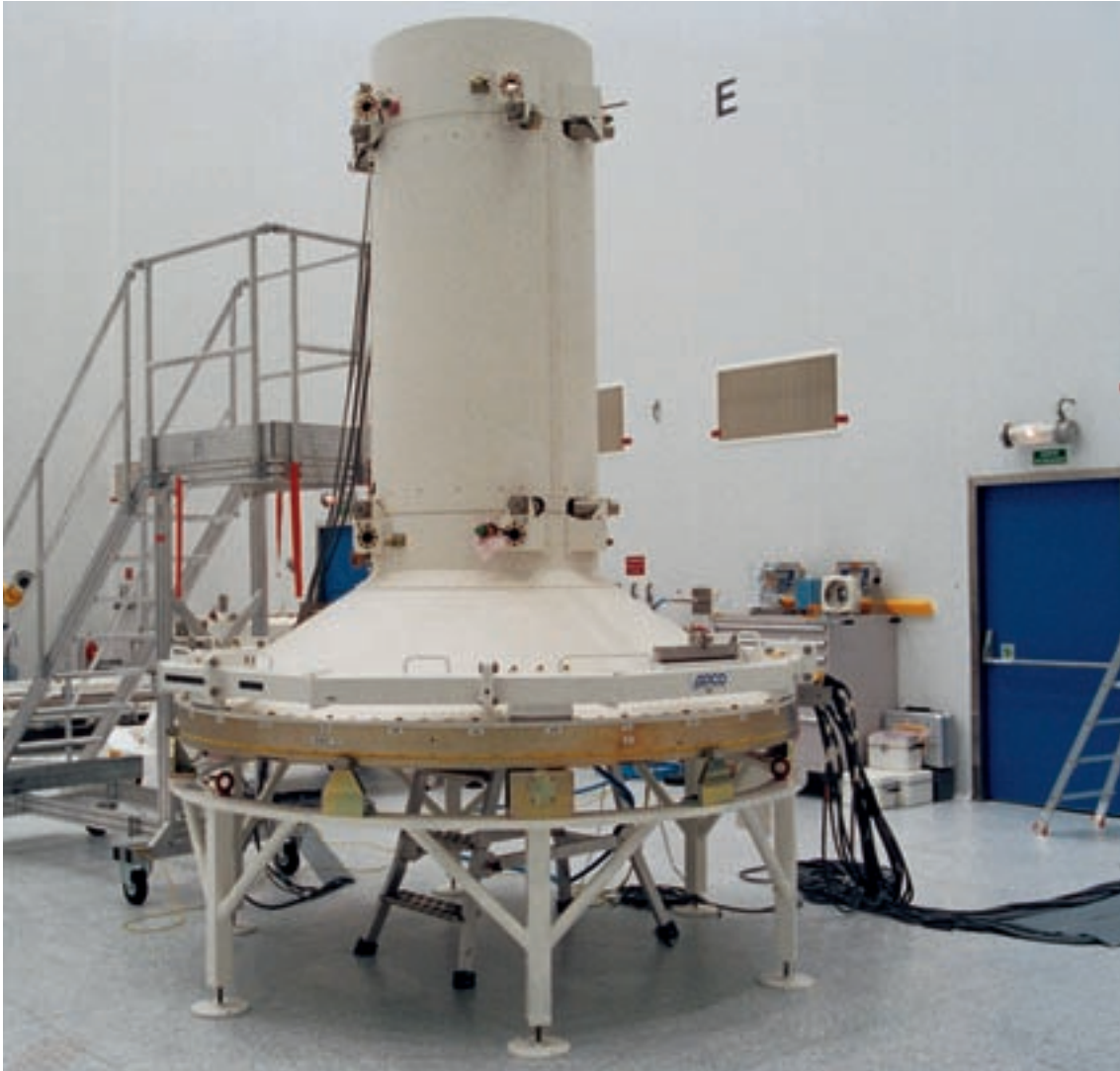
Figure A 2 - 11: GLS Dispenser on Its Integration Stand Prior to Spacecraft Mating (Hazardous Processing Facility)
