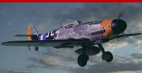
The main German fighters faced by the Tuskegee pilots were the Messerschmitt Me-109 Models "F" and "G". The Me-109G was powered by a 1,475 hp Daimler-Benz engine. It had a range of 435 miles (700 km) and a top speed of 400 miles per hour (640 km). It was armed with one 30mm MG FF cannon firing through the nose and two 13mm MG 131 machine guns firing through the propeller arc and two more 20mm MG151 cannons in the wings.
