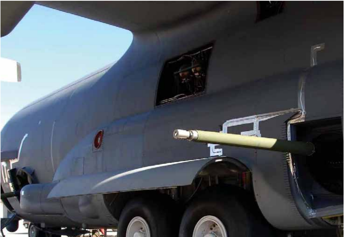
Bushmaster 30 mm cannons protrude from the gunports of an AC-130U Spooky gunship during tests at Hurlburt Field, Fla. The 30 mm gun will eventually replace both the 40 mm cannon and 25 mm gun on U-model gunships. Photo by Chief Master Sgt. Gary Emery.
