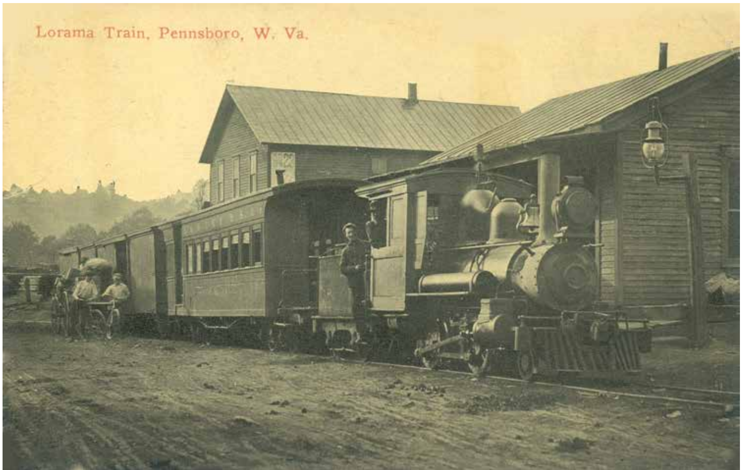
Lorama RR # 4 at Pennsboro, waiting for the box cars to be unloaded. The Lorama had two combines, an older model with seven round top windows and this one with eight straight top windows. Postcard from the collection of the author.
