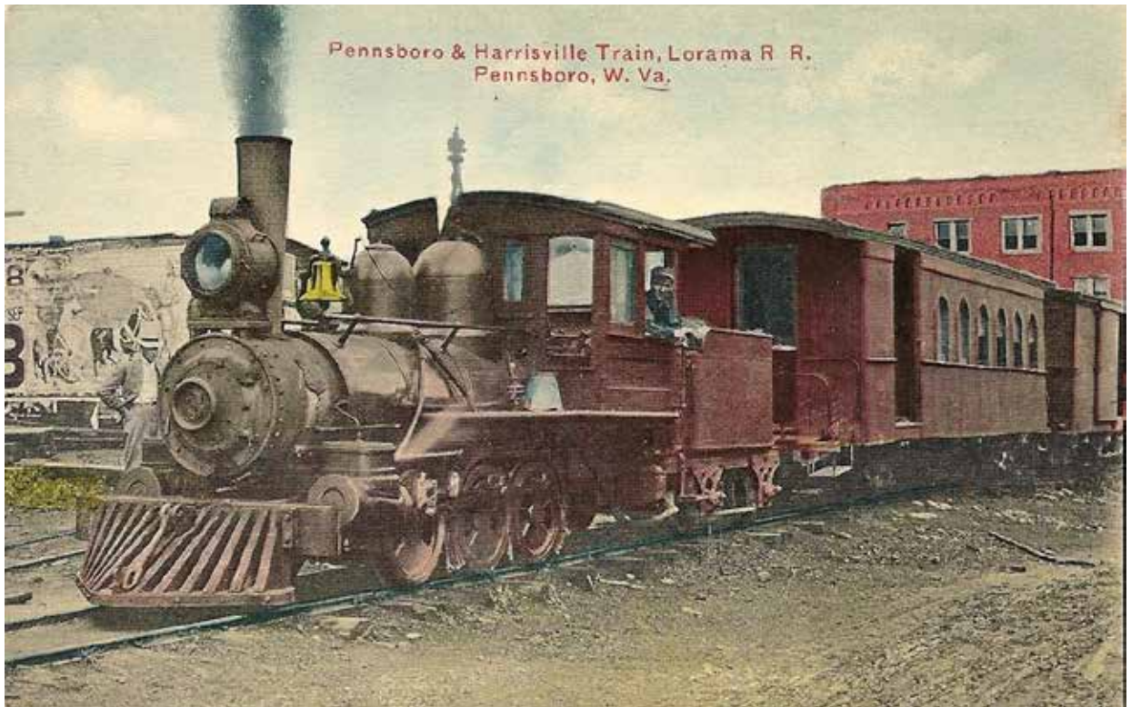
Lorama RR #3, a small Porter 0-6-0 with a four wheel tender and a mixed train in tow, prepares to leave the depot at Pennsboro, WV circa 1910 for its eight mile and 45 minute journey to Harrisville.. Postcard from the collection of the author.
