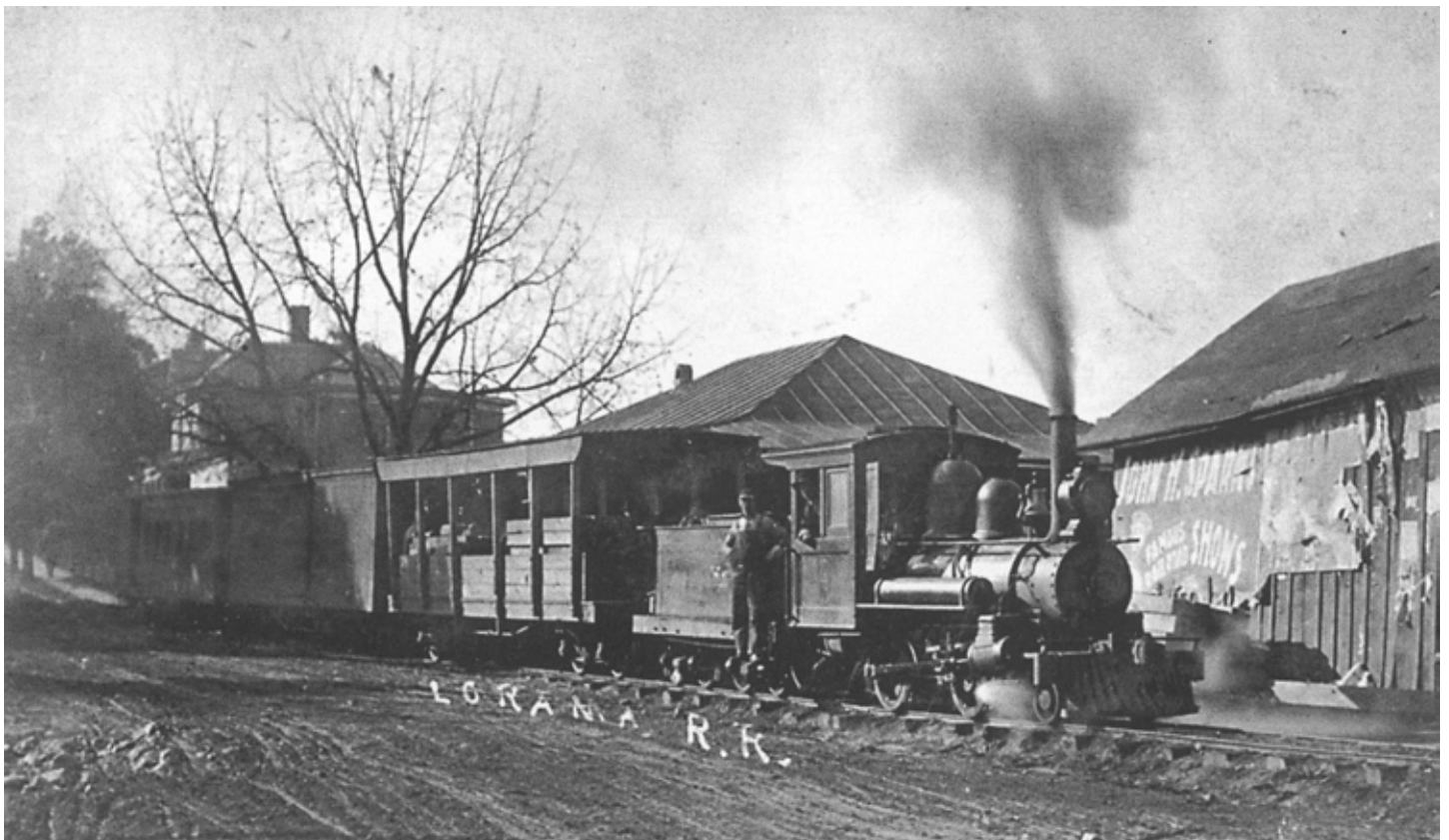
Lorama RR #4, a tiny Porter 2-4-0 with a four wheel tender and a mixed train in tow, prepares to leave the depot at Harrisville, WV circa 1916. One of the flat cars has been outfitted to excursion duty, so its possible this train was running during the Ritchie County Fair. Postcard from the collection of the suthor.
