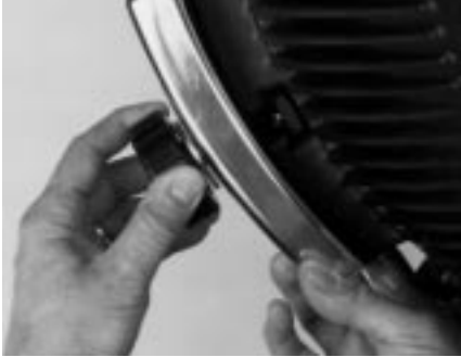
Figure 2 - Install clamps. Do not tighten yet.
