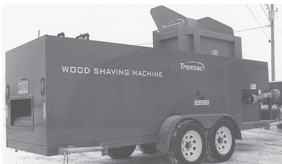
"It has a lot of capacity and works fast," says Bernie Riopel about his pto-powered shaving machine. It converts logs up to 22 in. dia. into wood shavings.
