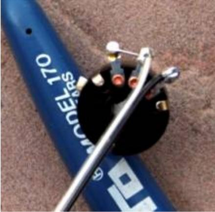
Figure 45. Prepare R88 100K Cw speed pot as shown. The left and middle terminals are connected to the white lead
