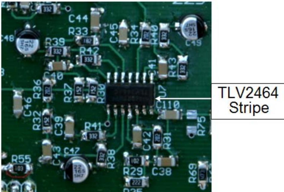
Figure 93. Component placement and alignment of U7 and polarization of caps C47, C48, C49
