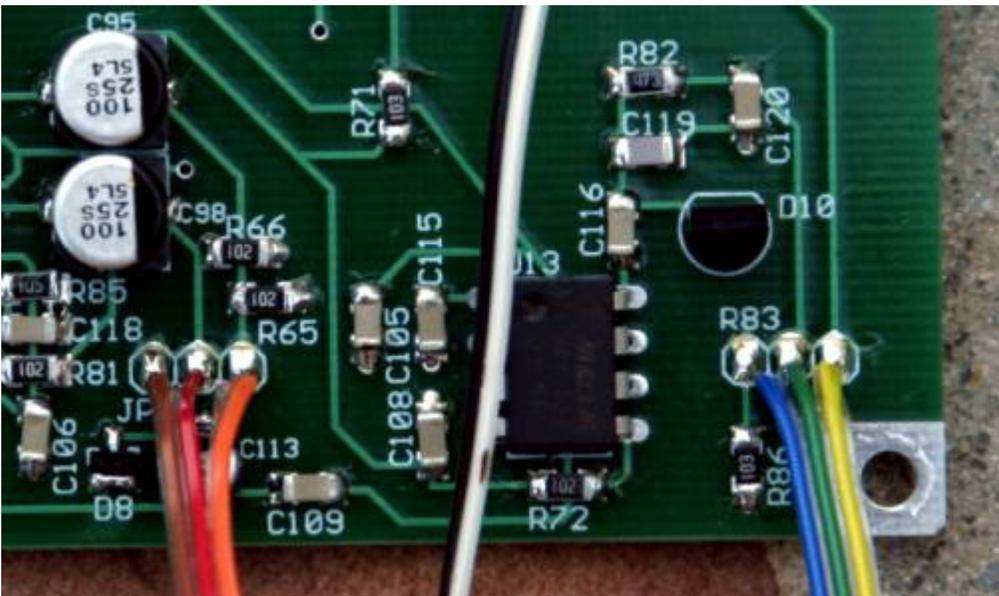
Figure 52. Connect the 50K SCAF pot to the R83 header pads in the color order shown
