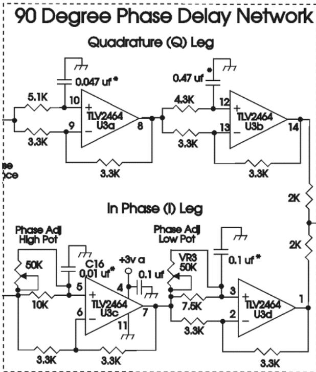
Figure 131. Audio phasing section schematic
