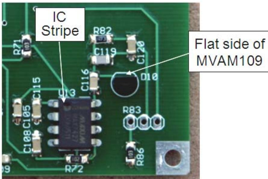
Figure 37. U13 and D10 mounted. IC notch and D10 flat side in the vertical direction.
