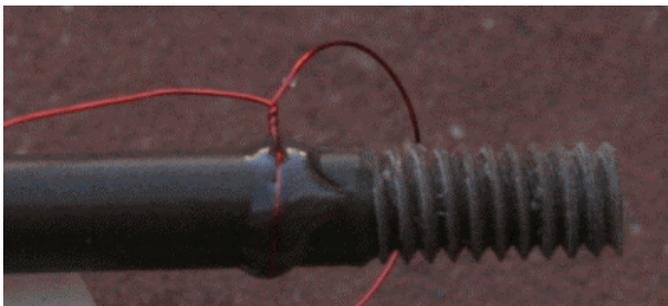
**Figure 74. First turn is glued (epoxy) into place to make it easier to wrap the rest of the turns**
