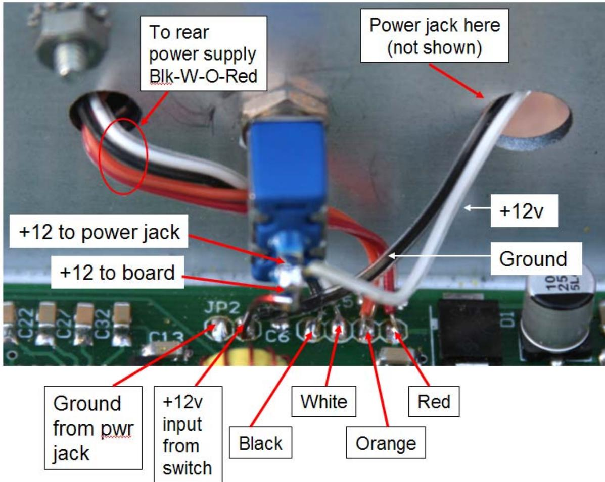
Figure 111. Rear power connections: Power switch, leads to rear switching supply, power jack (not shown)
