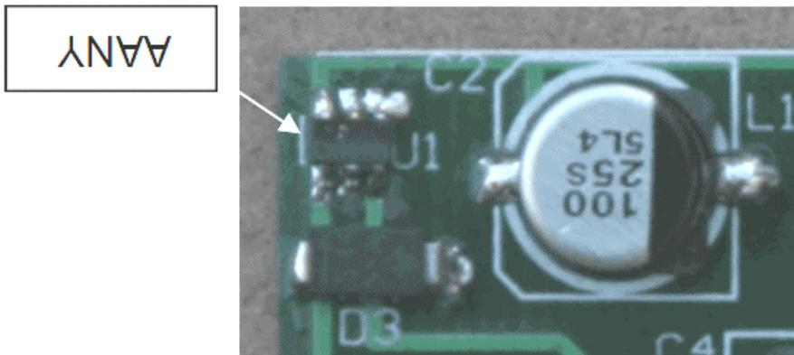
Figure 14. Orientation of U1. **Mount with the markings “AANY” upside down as shown.**
