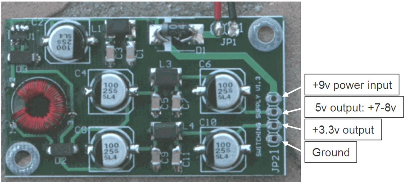
Figure 23. Power Output Connection Details (Load resistor not shown)
