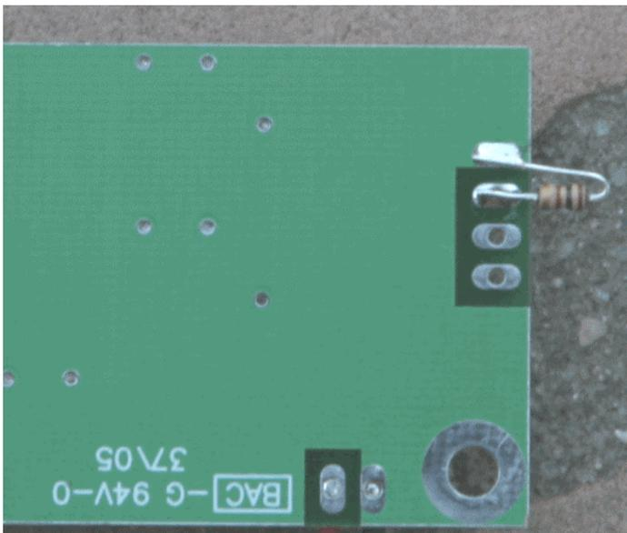
**Figure 22. 3v Temporary 100 Ohm Load Resistor Connected to Bottom of Board**
