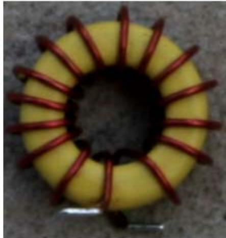
Figure 82. Coils L6 and L7 are prepared to be mounted surface mount style on the top of the board on the coil holes
