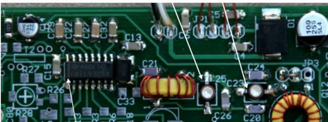
Figure 126. Location of RF front end band pass filter adjust trim caps, C23 and C25 on top middle of the board
