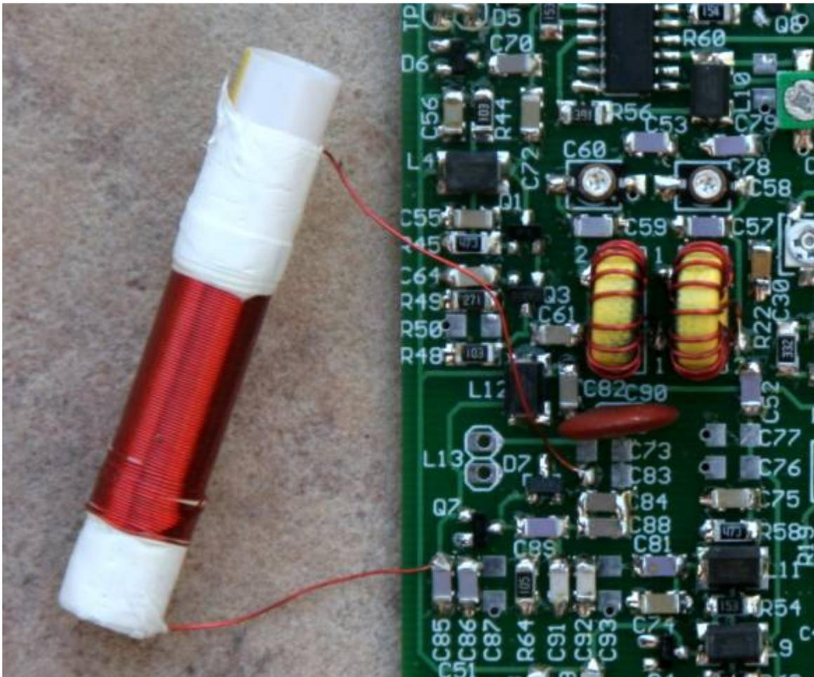
Figure 68. Temporary soda straw PTO coil L13 connected to the PTO oscillator circuit.
