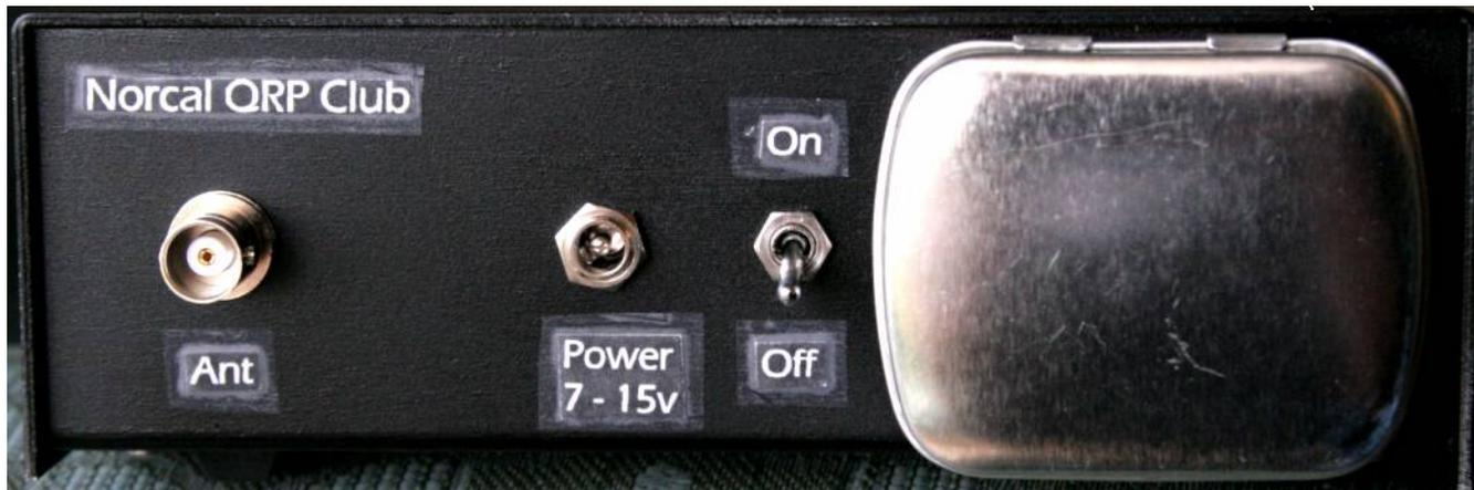
Figure 109. Rear panel of prototype NC2030. Final case will be silk screened.
