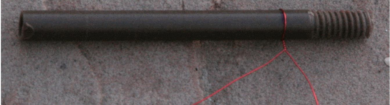
**Figure 73. Wrap first turn on the PTO coil. Position  $\frac{3}{4}$ ” back from front, twist single turn in place**
