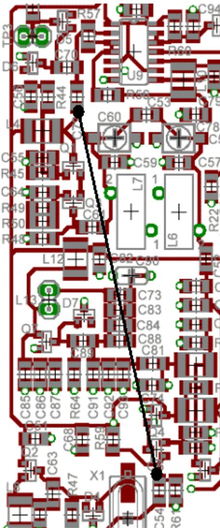
Figure 64. Temporary connection from C72 to C54
