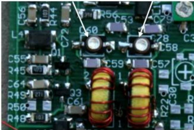
Figure 81. LO Filter and amplifier as built. Both trim caps must have proper orientation
