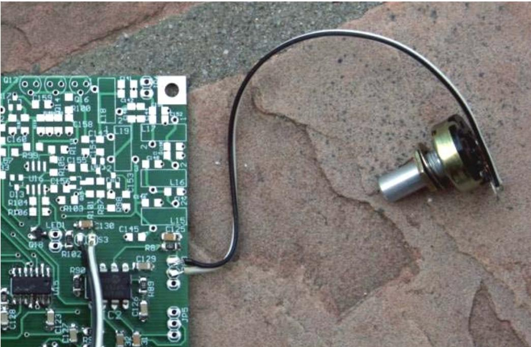
Figure 46. Connect R88 CW speed pot to the R88 pads as shown. Keep black and white in order shown.
