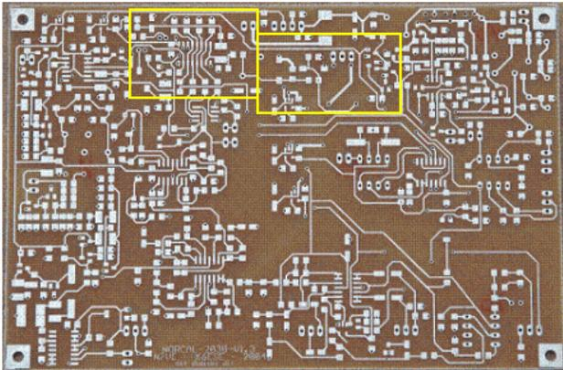
**Figure 83. General location of the Detector and Front End Filter**
