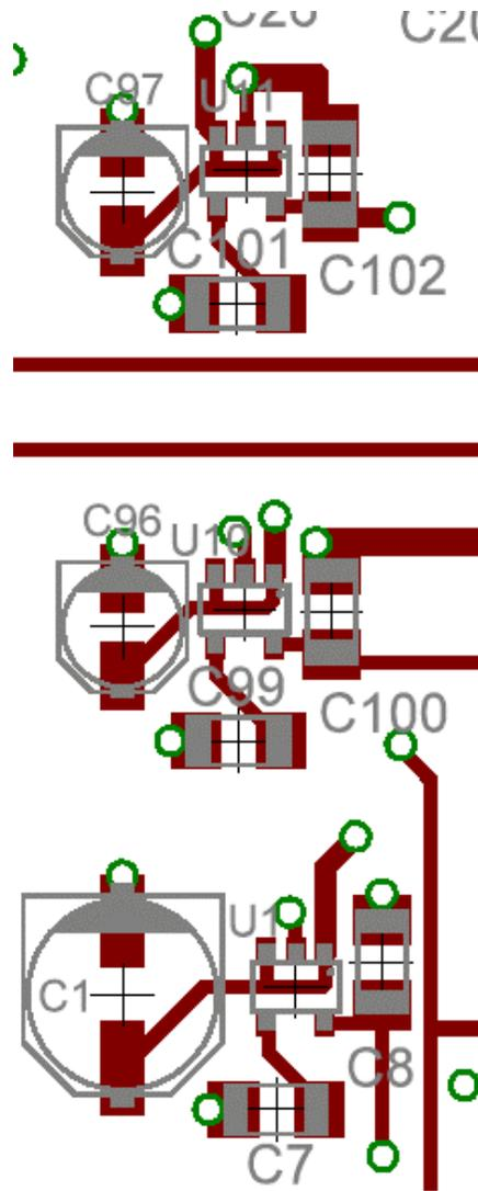
**Figure 29. Location of the one 3v and two 5v LDO regulator sections**
