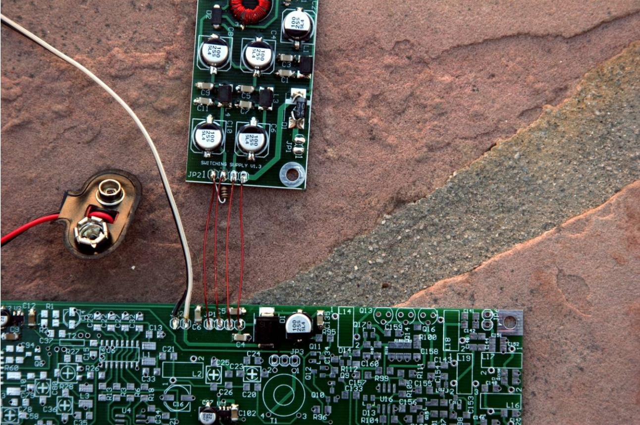
**Figure 24. Temporary 9v power connection and connections between switching supply and main board**
