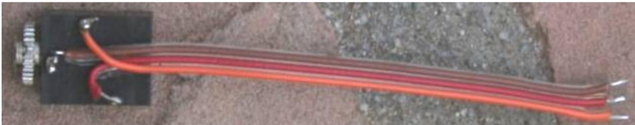
**Figure 49. Use Brown/Red/Orange wire and connect up the headphone jack in the color order shown**
