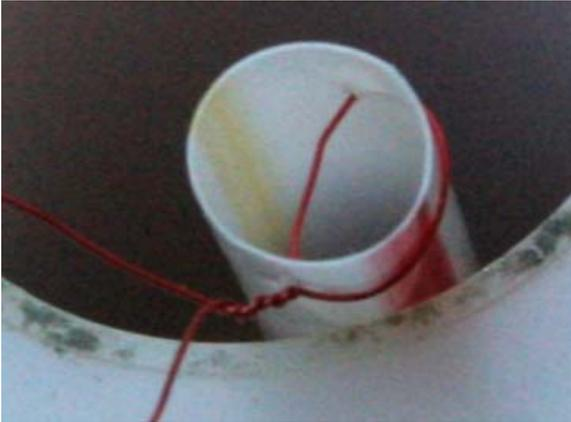
**Figure 69. Anchoring the first turn of the temporary PTO coil.**
