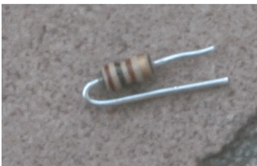
**Figure 20. 100 ohm Temporary 3v Load Resistor Formed as Shown**
