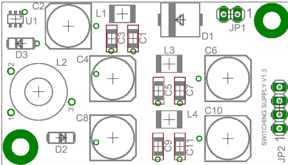
Figure 12. Board layout of the switching power supply.
