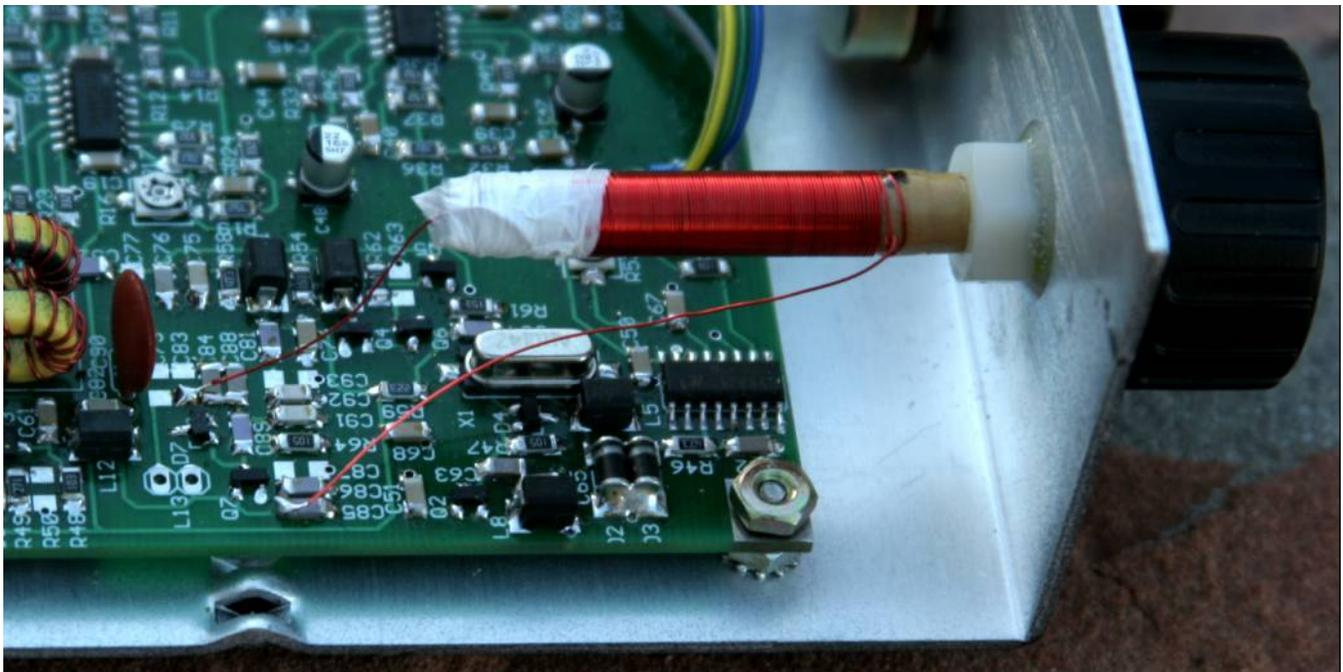
Figure 116. PTO L13 mounting detail. Coil connections shown. Front PTO coil wire must connect as shown.
