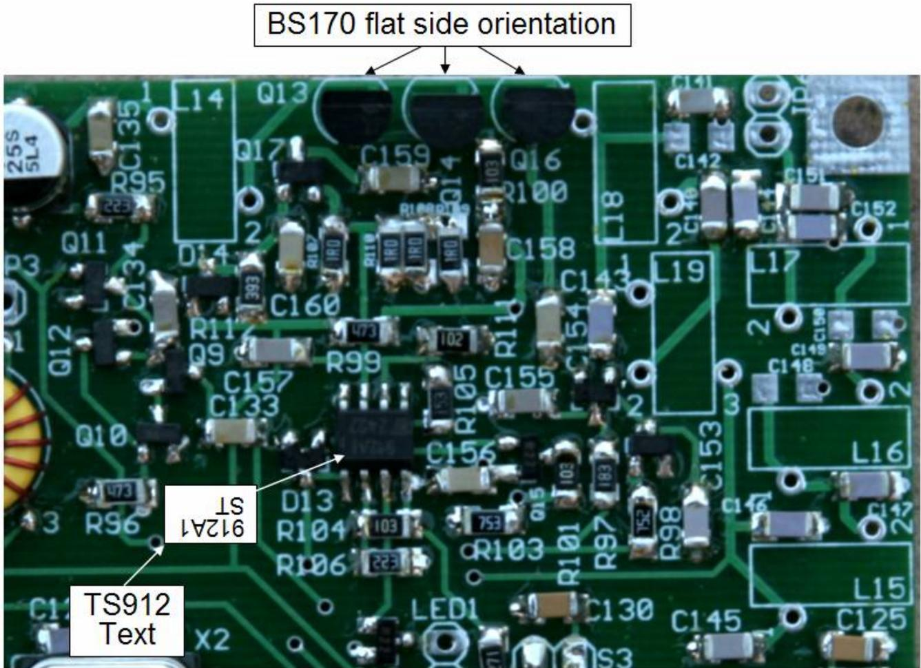
Figure 96. All transmitter parts except for the inductors. Note TS912 orientation, BS170 flat side orientation.
