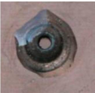
Figure 118. Front side of the PTO coil (prototype chassis) showing epoxy ridge from the front side
