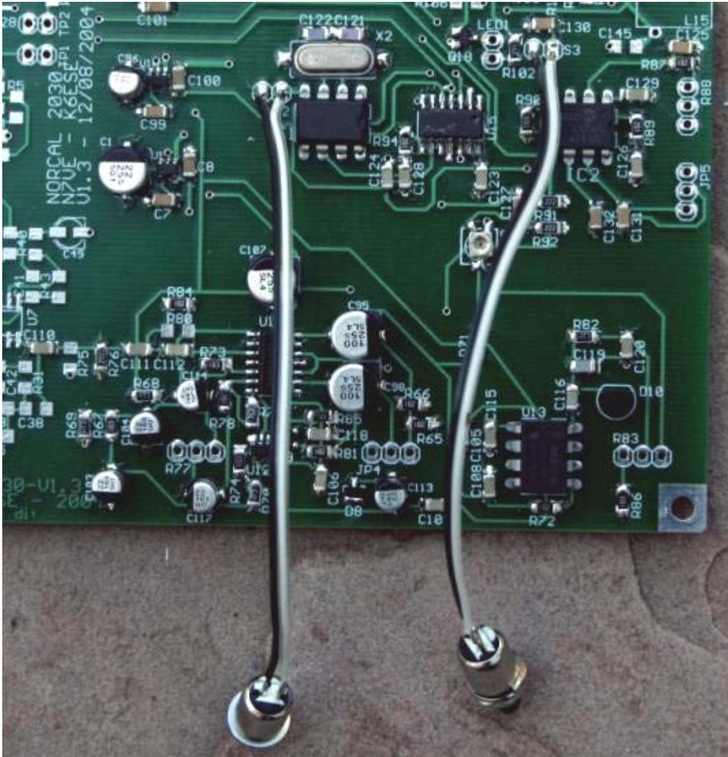
Figure 44. Connect buttons keyer and AFA buttons S2 and S3 as shown
