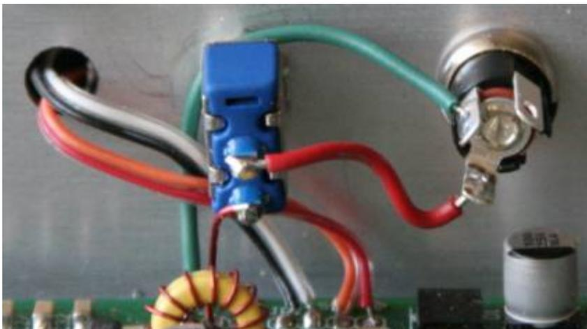
Figure 112. Power jack connections, +12v to power switch (red wire) and ground (green) to JP2 ground pad
