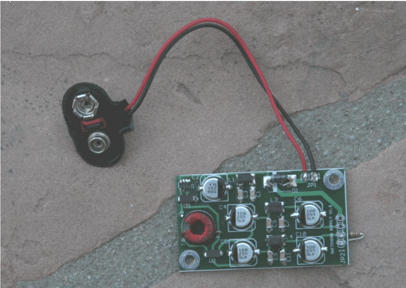
Figure 11. Completed Switching PS with Temporary 9v Power Connection and 100 ohm 3.3v Dummy Load
