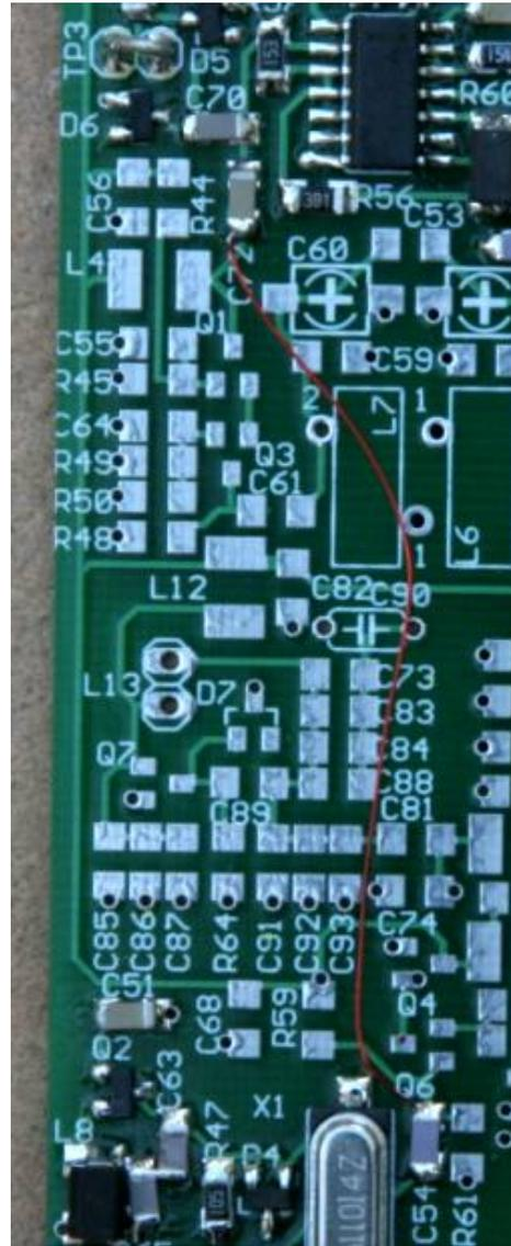
First install a temporary wire connection from C72 to C54 as shown above. Use a short length of # 32 gauge enamel wire to make the connection. This connection will allow the SSS AFA to measure the frequency of the VXO.
