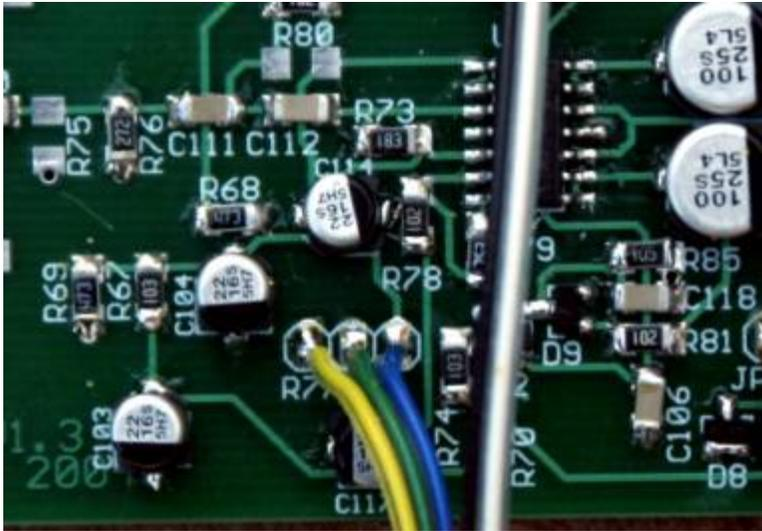
Figure 54. Connect the 5K volume control pot to the R77 header pads in the color order shown
