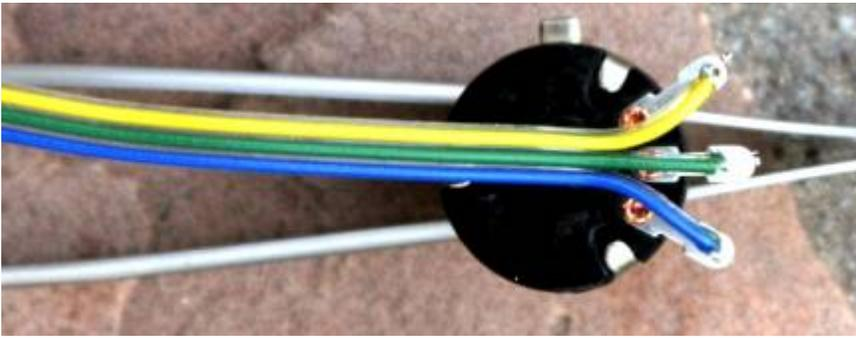
Figure 51. Use Yellow/Green/Blue wire to connect to R83, the 50k SCAF pot in the color order shown
