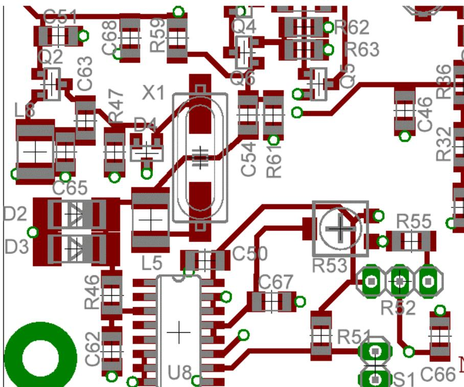
Figure 57. Close up of VXO and T/R offset circuit
