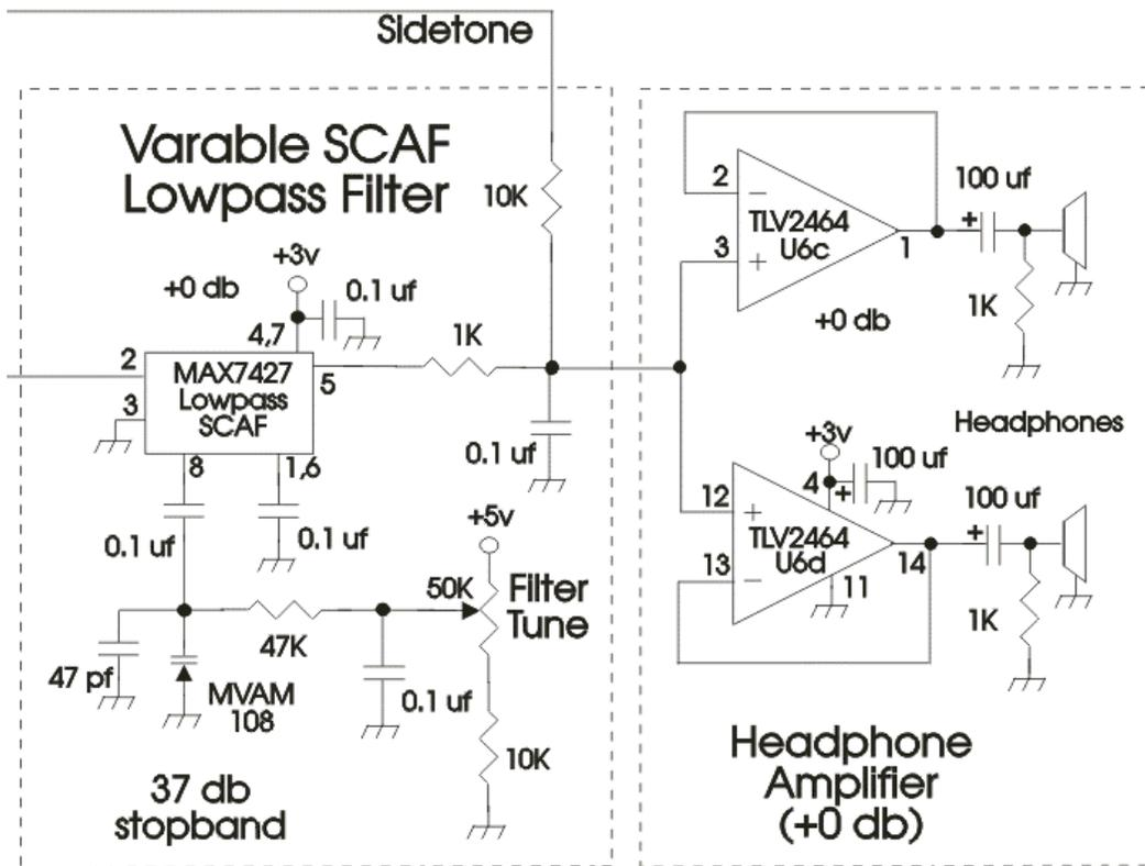
Figure 134. SCAF Low Pass Filter and Headphone Amplifier
