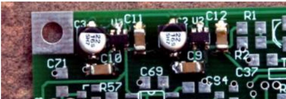
Figure 28. Parts layout of first two 2.9v LDO regulators. Note the black band orientation of the electrolytic caps.
