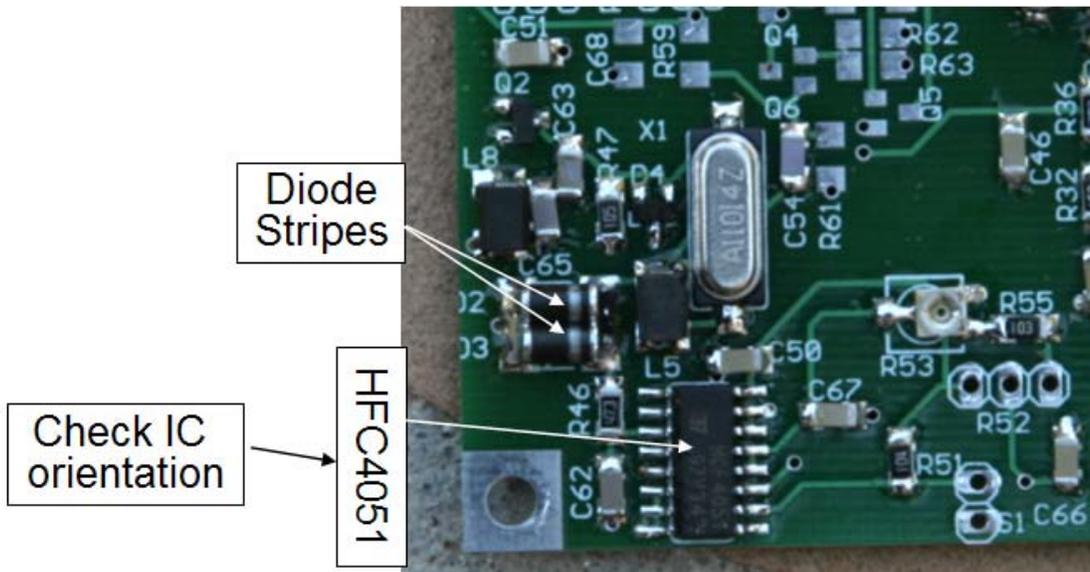
Figure 58. Proper orientation of U8, D2, and D3
