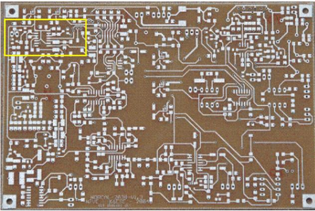
Figure 61. General location of the AFA RF Buffer and Phase Splitter
