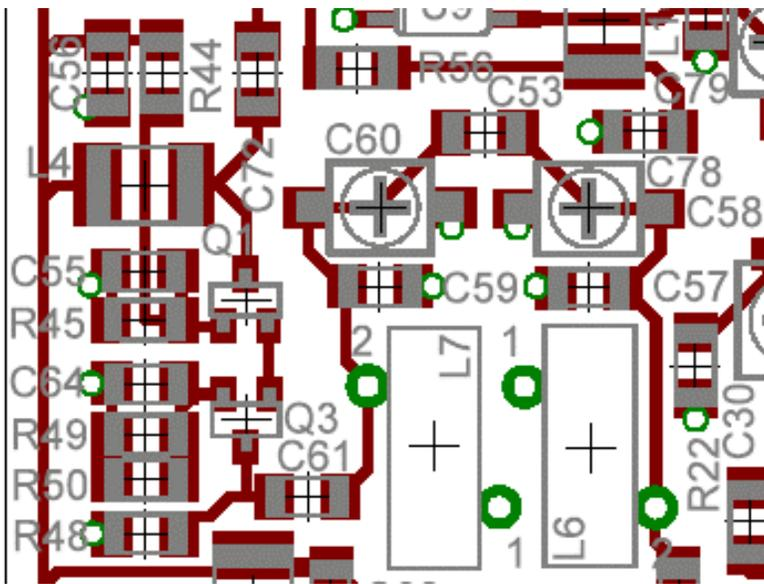
Figure 80. Close up of the LO Filter and Amp components
