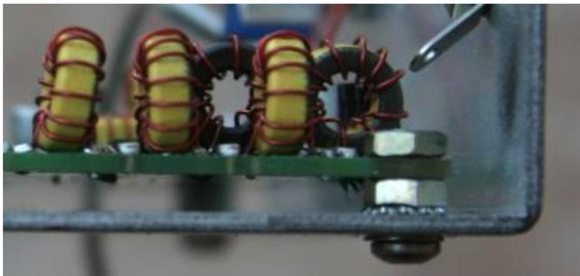
Figure 101. Mount all four corners of the main board using the mounting hardware as shown.
