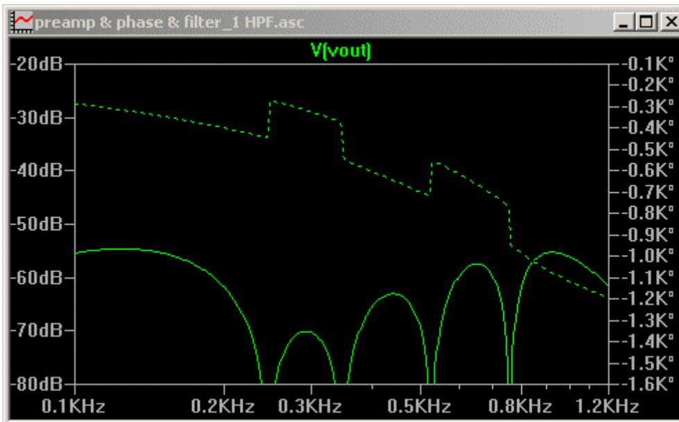
Figure 128. Picture of simulated opposite sideband rejection when optimally tuned up.
