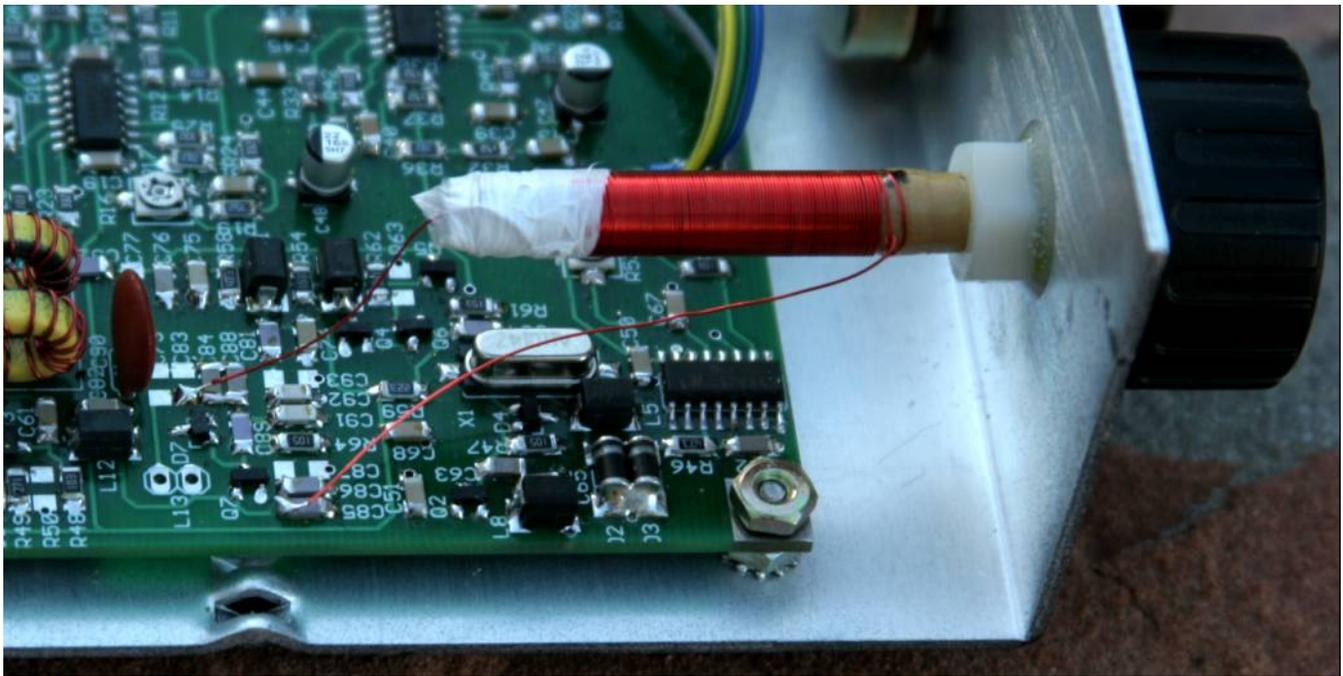
Figure 72. Main tuning PTO coil L13 shown mounted to the front panel. This is used only when the rig is finished.
