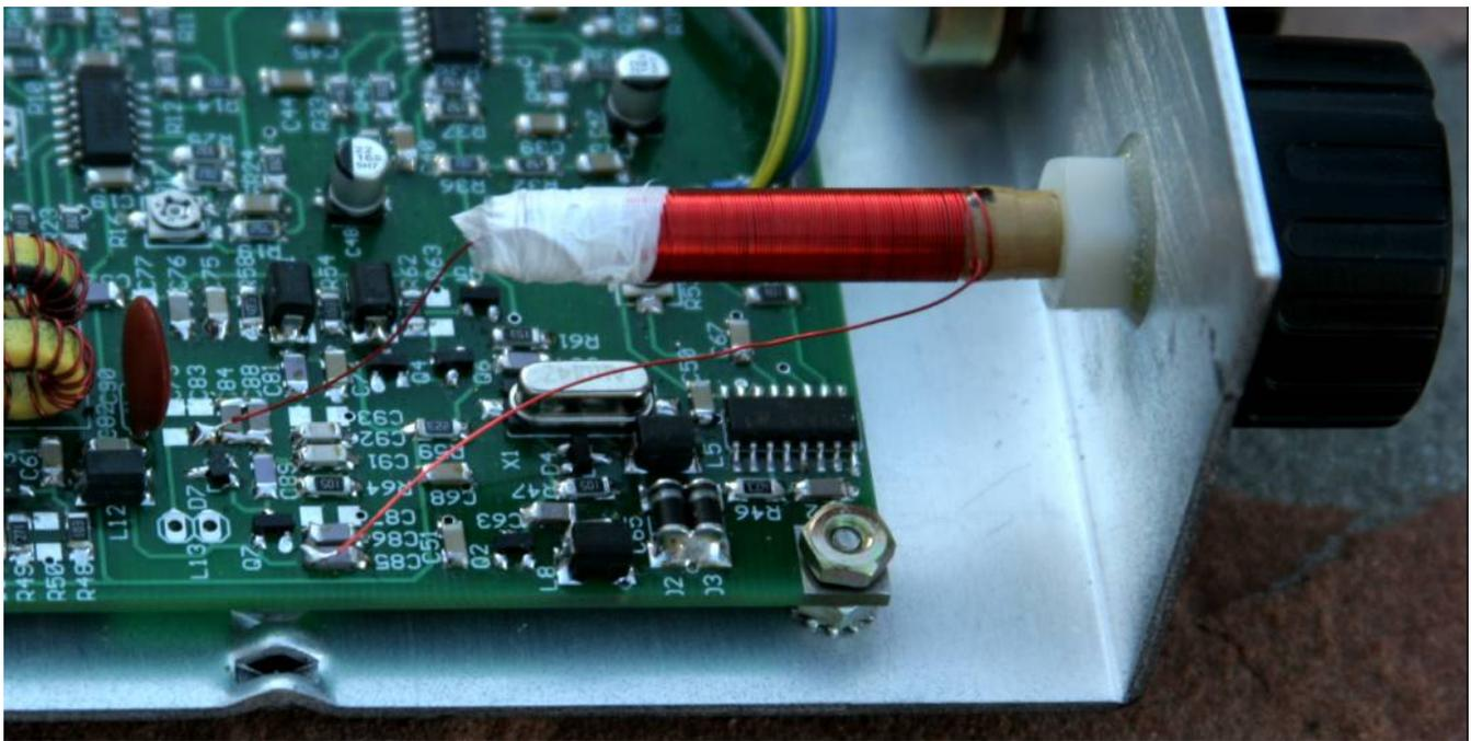
Figure 123. L13 PTO tuning coil as mounted. Remove turns off the end simply by pulling on the wire.
