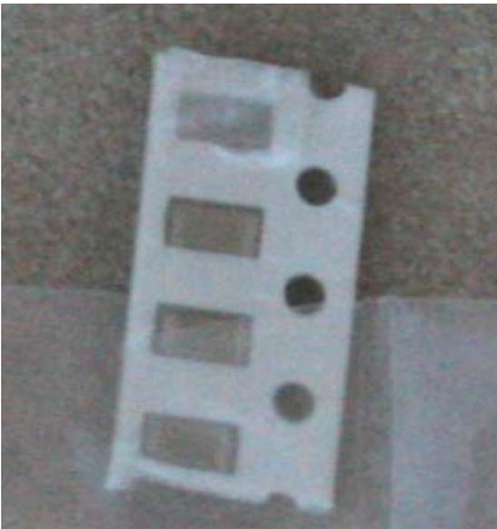
**Figure 6. Close up of a surface mount parts strip and the bag slit just large enough to access the strip.**
