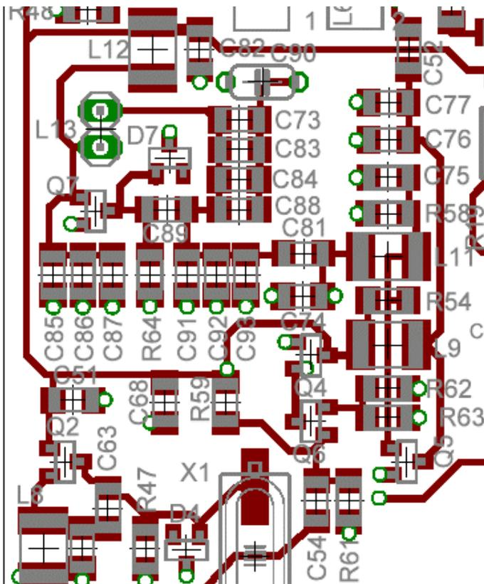
Figure 66. Close up of the PTO and Mixer section of the board
