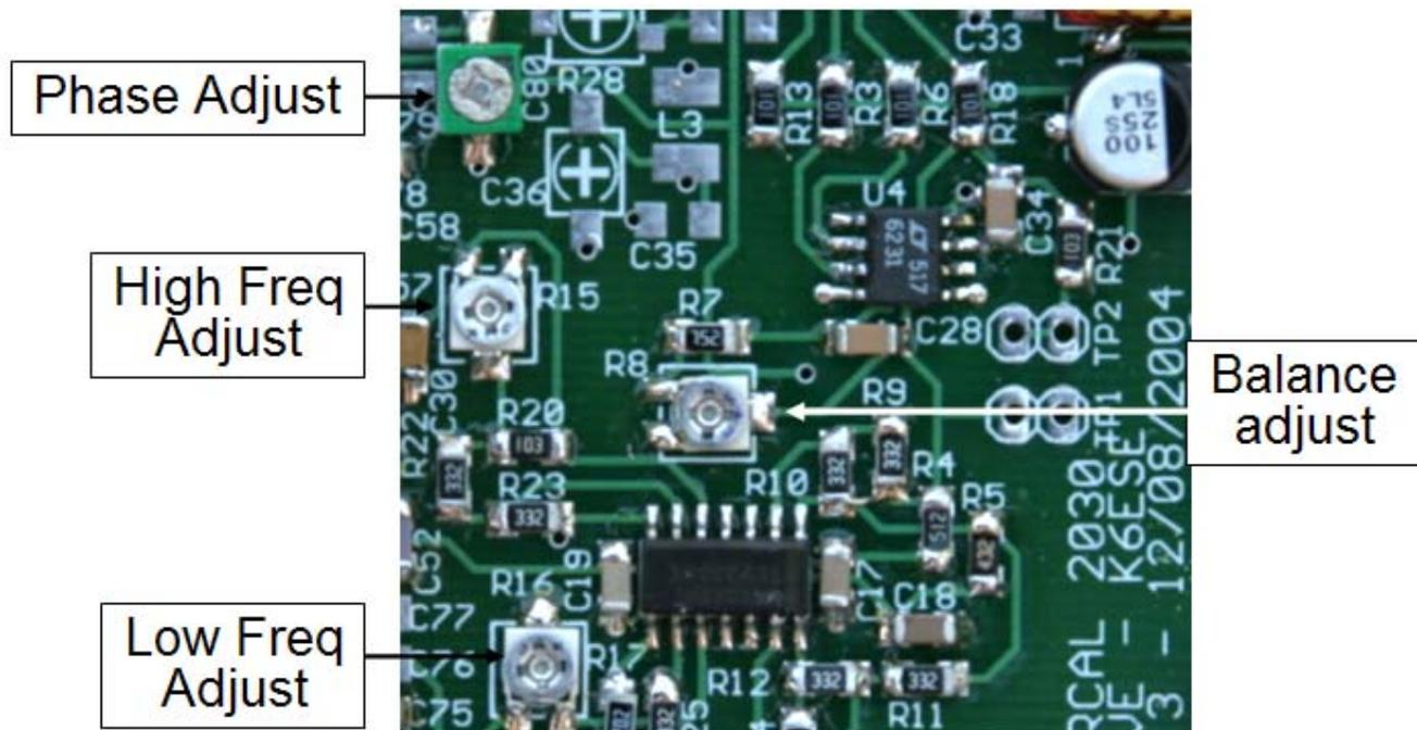
Figure 127. Adjustment points for nulling out the opposite sideband
