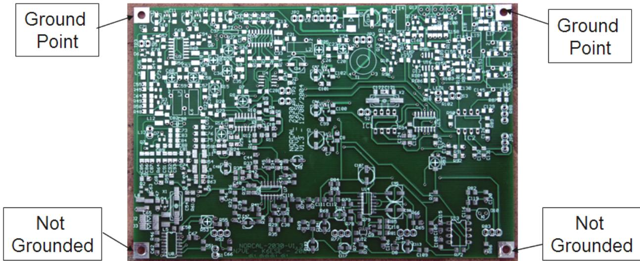
Figure 31. Ground reference for voltage measurements are upper 2 corners, the lower 2 are not connected
