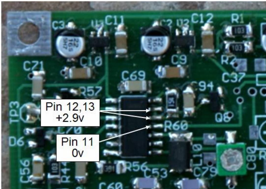
Figure 98. Location of U9 and pins voltages to check. In receive mode, check, U9 pins 11 (0v), 12 &13 (2.9v).
