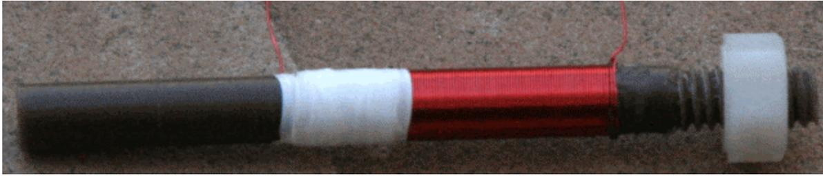
**Figure 75. Coil with completed 105 turns. Turns wound tight and “shoulder to shoulder”.**
