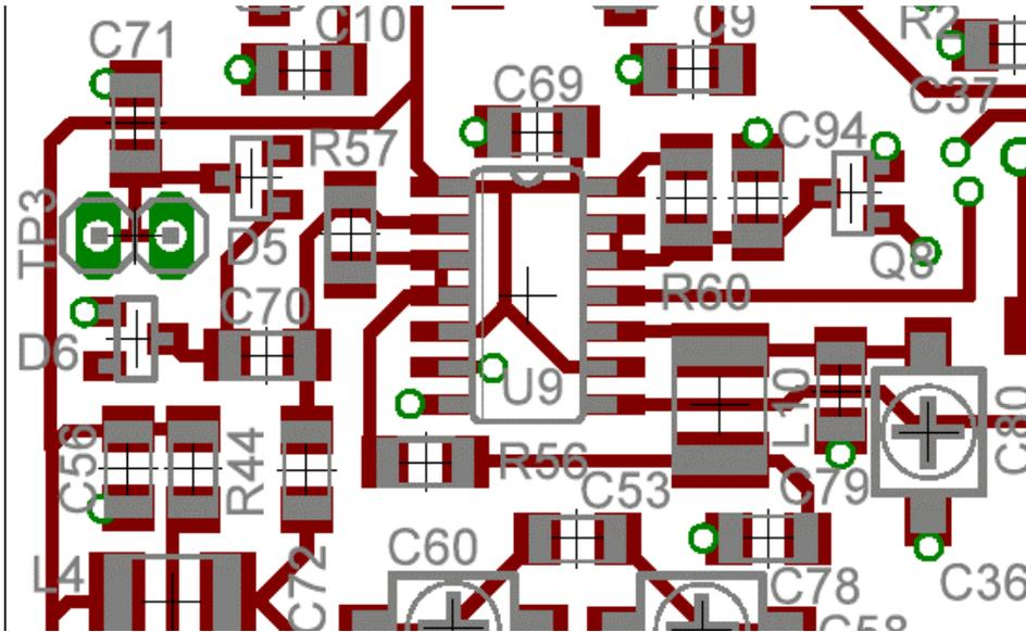
Figure 62. Close up view of the AFA RF Buffer and Phase Splitter Area
