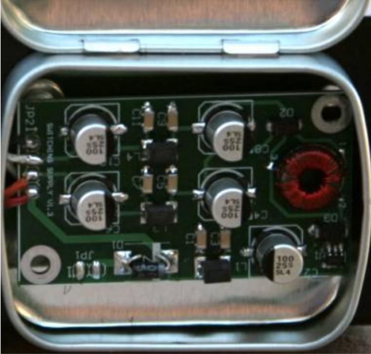
**Figure 114. Place the switching supply board in the tin, center it top & bottom, and mark the mounting holes**
