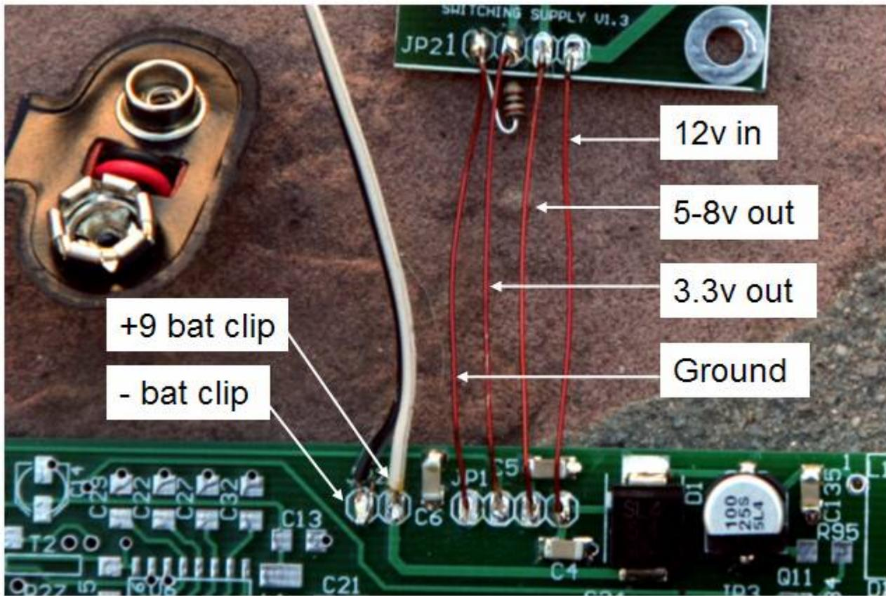
Figure 25. Close up of power connections on the main board and switching supply, bypass caps, and polarity diode
