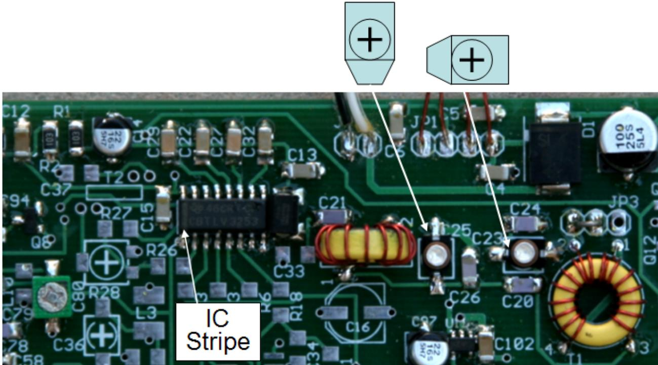
Figure 85. Picture of detector and RF front end with parts installed. Note trim cap orientation and jumper on JP3!
