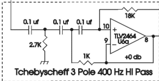
Figure 133. 400 Hz High pass filter schematic
