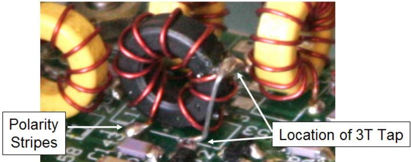
Figure 97. L19 mounted. 3T tap location shown.
