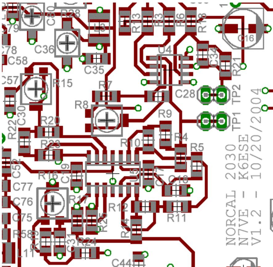
Figure 89. Close up of Audio Preamp and Phasing sections
