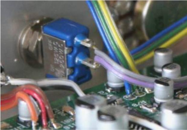
**Figure 107. Another view of the spot switch. The two terminals are orientated in the “up” position.**
