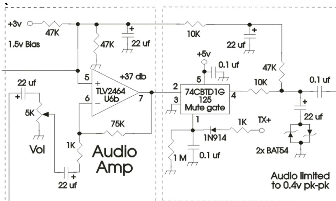
The amplifier stage has a gain of 75x (37 db) as set by the 75K feedback resistor and the 1K input resistor. The 1.5v bias at the + input to the amplifier is also used to bias the 400 Hz HPF above. This stage includes the volume control to set the listening level of the receiver.
