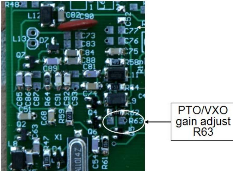
**Figure 124. Location of R63, PTO/VXO mixer gain adjust located in bottom left corner of board**
