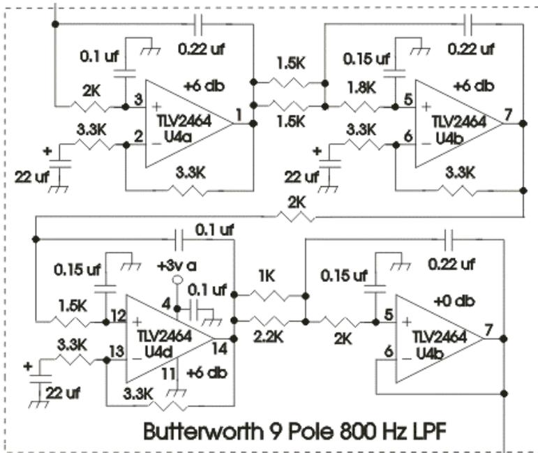
Figure 132. Main brick wall filter. 800 Hz active R/C low pass filter.
