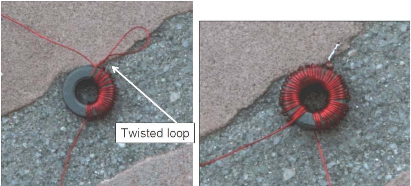
**Figure 18. L2 details. After first 24 turns, add a twisted loop for later center tap. Add 27 more turns after this.**
