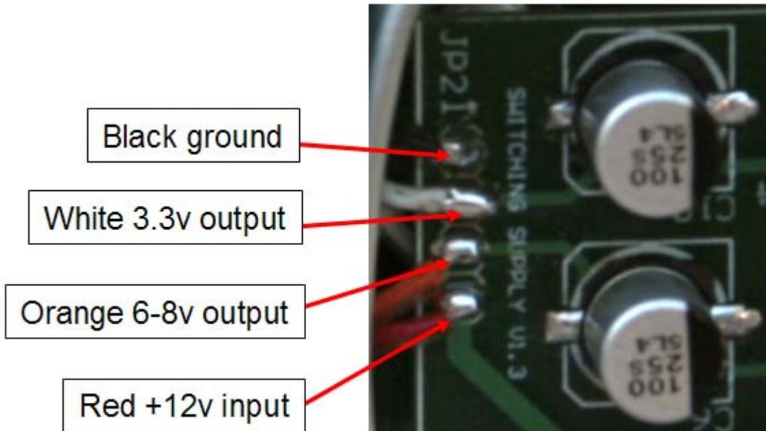
Figure 115. Connect the power wires to the switching supply in the color order shown.
