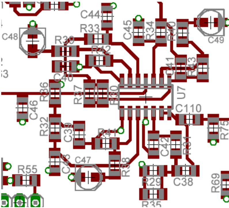
Figure 92. Close up of the 750 Hz Audio LPF section
