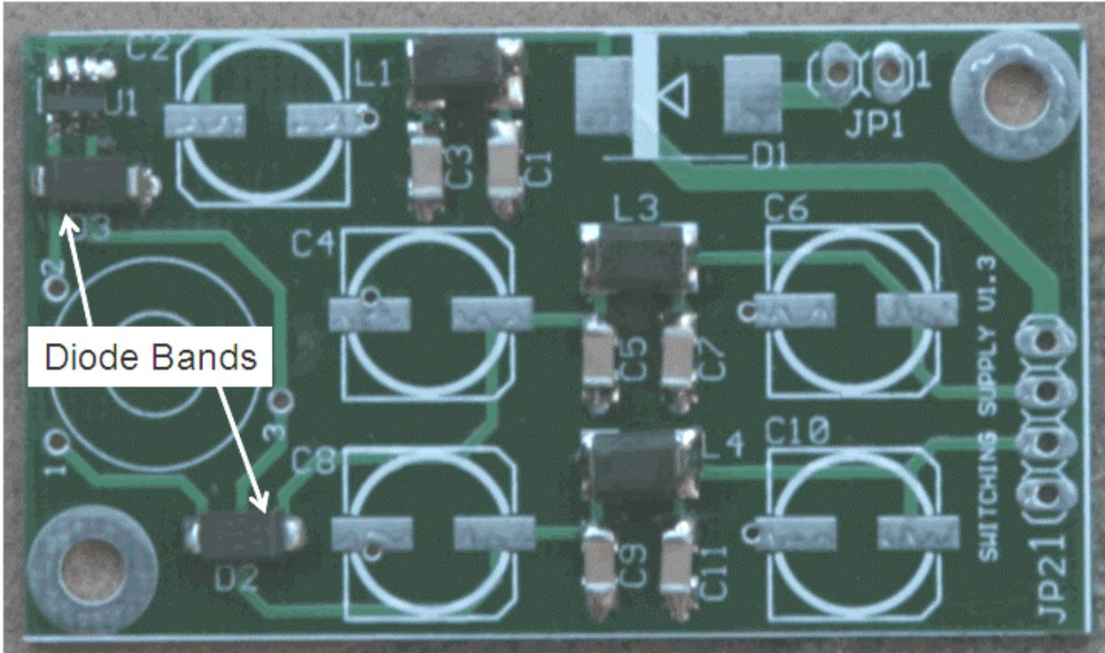
Figure 15. PS with 0.1 Caps, 47 uH inductors, Schottky diodes, and Switching IC
