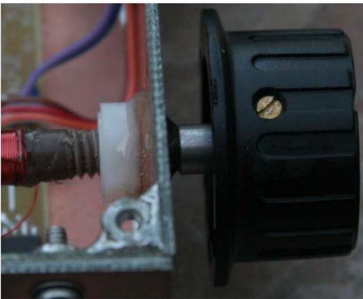
Figure 120. PTO brass screw full inserted into the PTO coil
