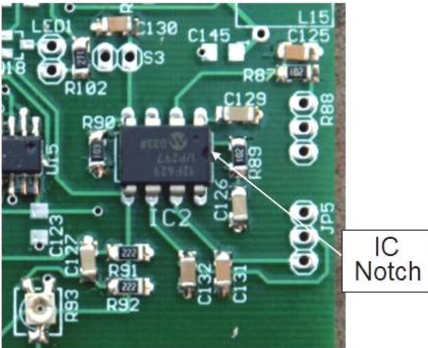
Figure 40. Picture showing correct orientation of Norcal Keyer Chip (optional socket not shown)
