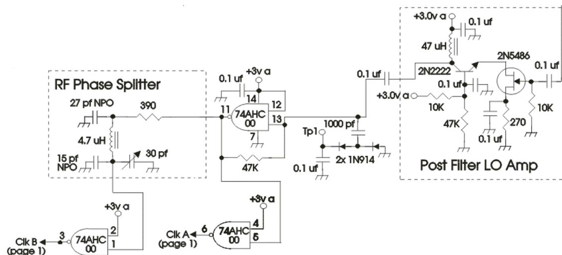
Figure 138. Schematic of LO amplifier and detector clock phase splitter
