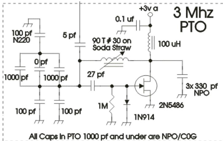
Figure 135. PTO schematic
