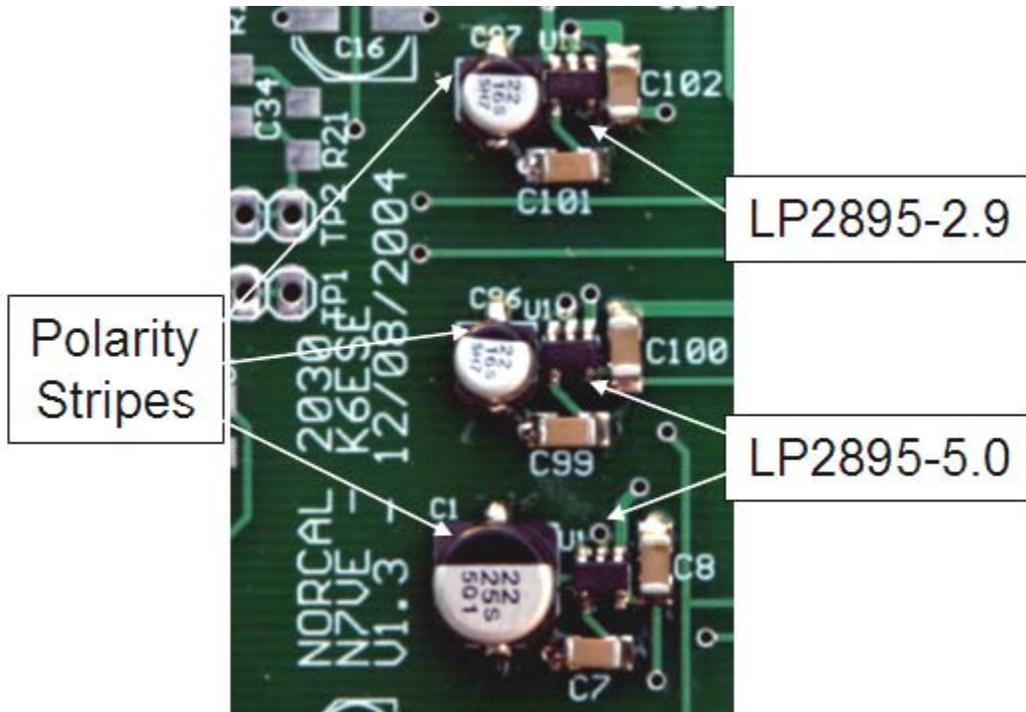
**Figure 30. Installed parts for this section of LDO regulators. Note the black band orientation on the electrolytic caps.**
