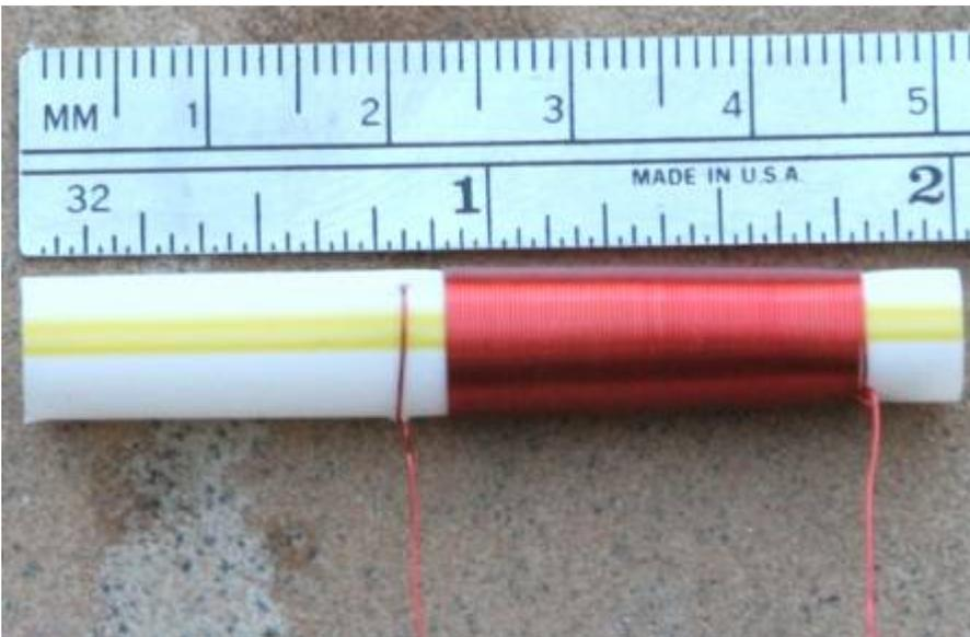
**Figure 70. Finished temporary PTO coil with 82T. Tie off holes placed on both ends**
