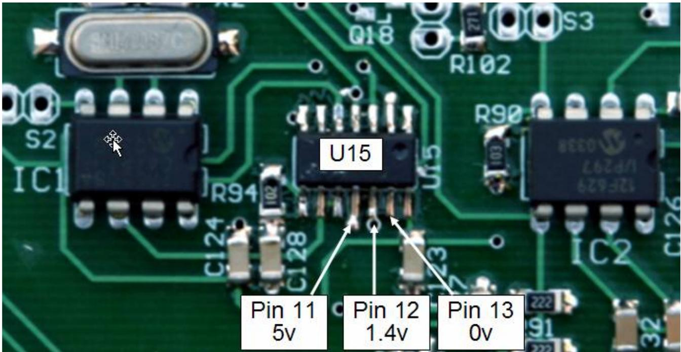
Figure 99. Location of U15 between AFA and Keyer chips. Test pins 11, 12, and 13
