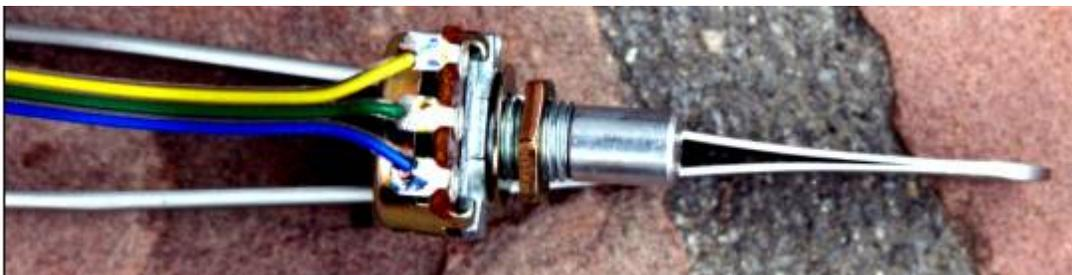
Figure 53. Use Yellow/Green/Blue wire to connect to R77, the 5K volume control pot in the color order shown
