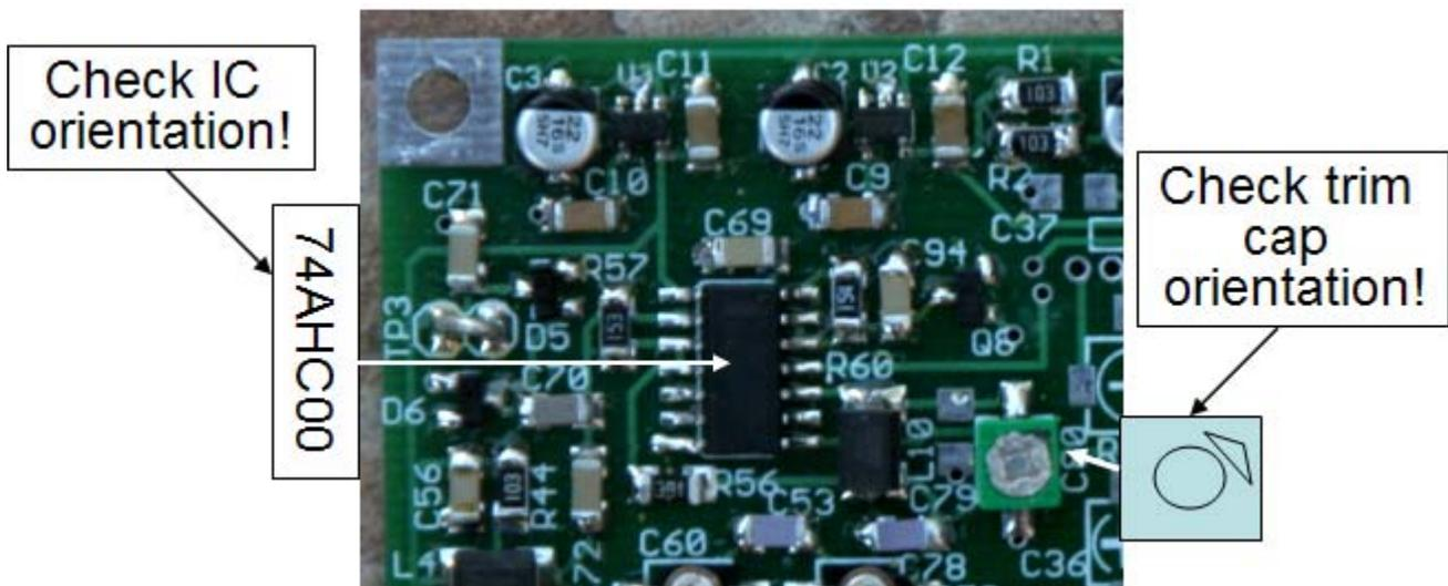
Figure 63. Orientation of U9 labeling as installed.
