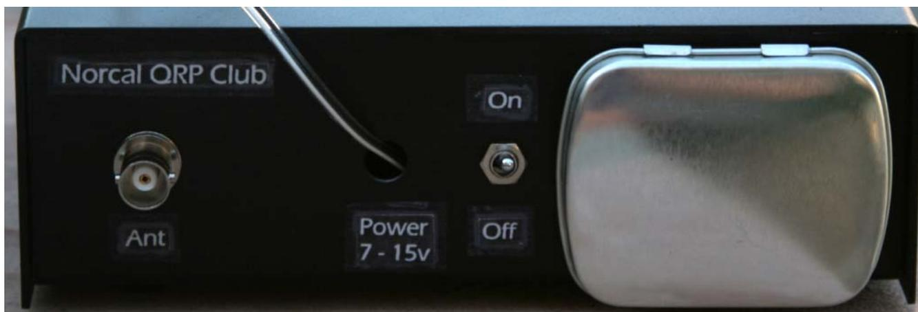
**Figure 113. Placement of the switching supply tin on the back chassis, power jacking not installed.**
