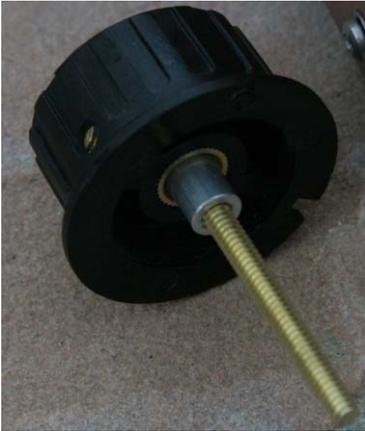
Figure 119. Tuning knob with PTO screw partially inserted.
