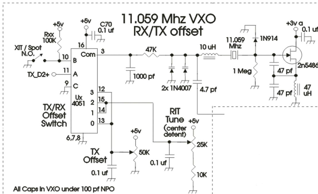
Figure 136. VXO schematic and transmit/receive offset switching
