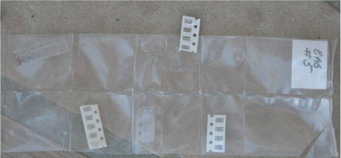
**Figure 5. Parts in bag pockets are accessed via slit cut into the packet just larger enough to get the part out.**
