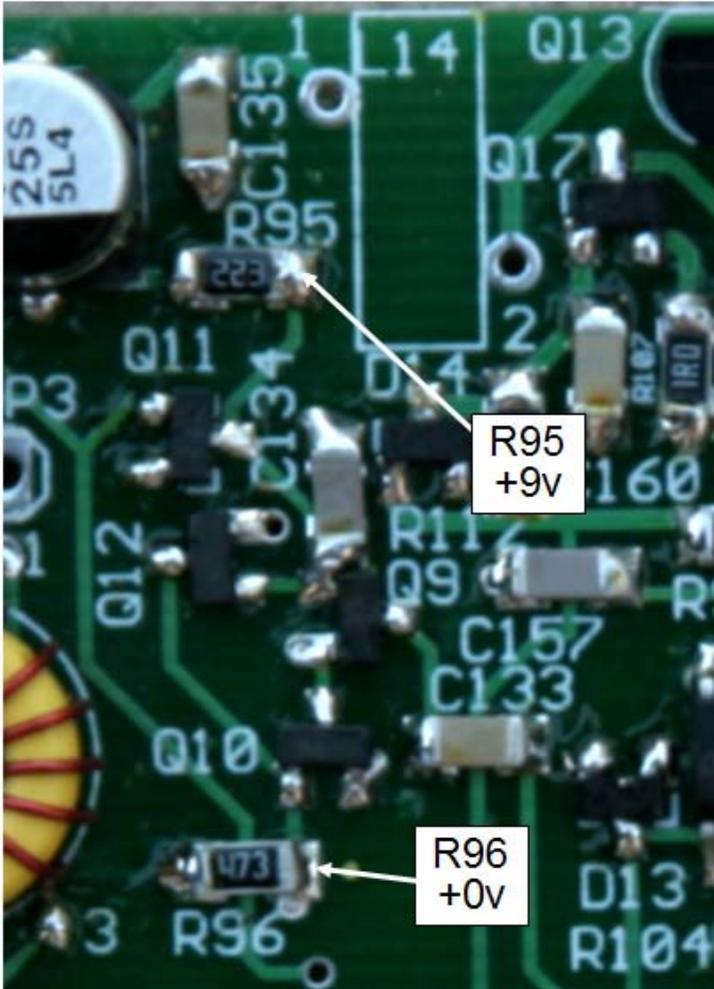
**Figure 100. Location of R95 and R96. Voltages on transmit/receive switches**
