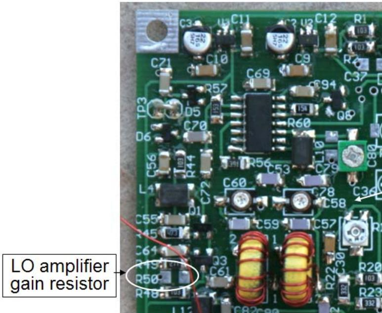
Figure 125. Location of optional LO amplifier gain adjust resistor R50
