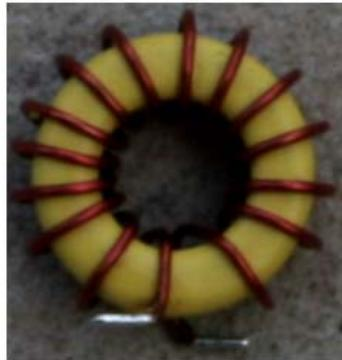
Figure 87. L2 leads formed to prepare for surface mounting on the top of the through hole pads provided.
