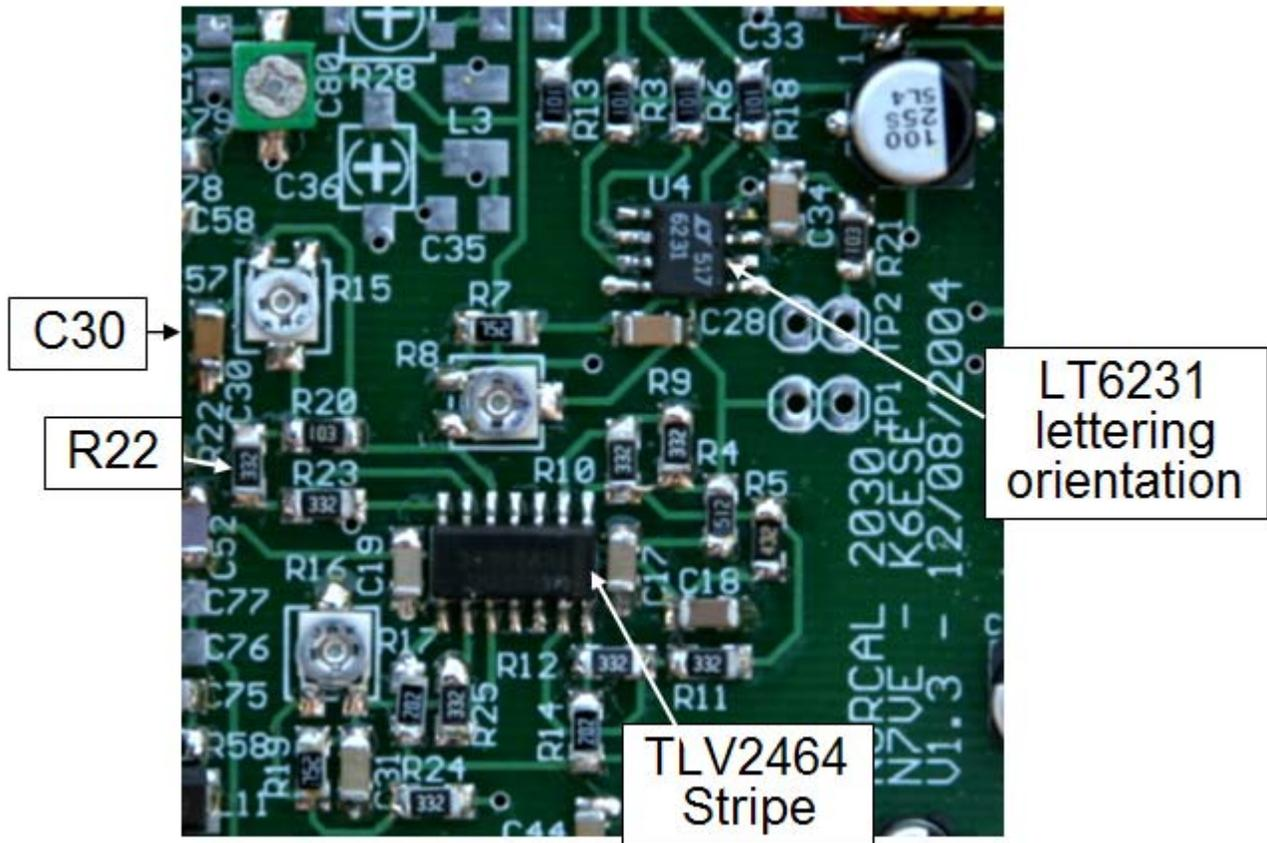
Figure 90. Component alignment of U4, and U5. Note C30, R22 locations
