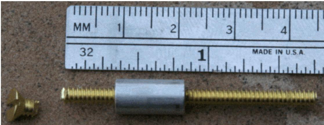
Figure 77. 2" brass screw cut back to a total length of 1 3/4 inches.
