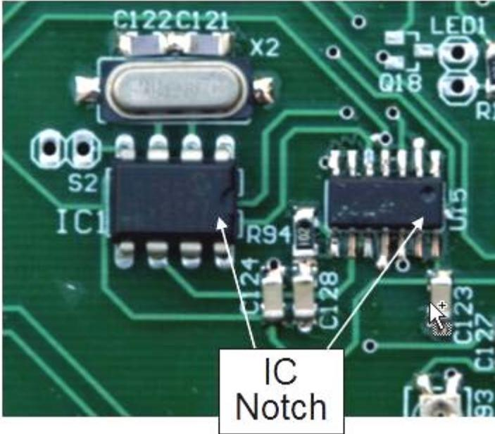
Figure 43. Correct orientation of both the 8 pin 12C508 AFA chip and 14 pin 74ACT00 ICs.
