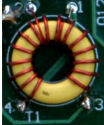
Figure 86. Detail on T1. Two turn # 32 to pads 1 & 2. Main winding connect to pads 3 & 4.
