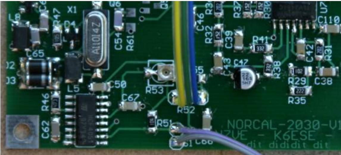
Figure 60. Connect the 25K RIT pot to the R52 header in the color order shown. Also attach a SPDT switch to S1
