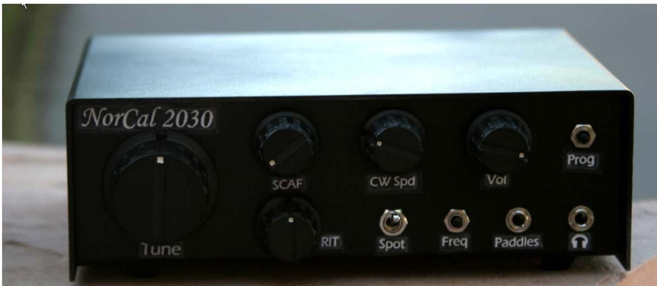
Figure 102. NC2030 with all front panel hardware mounted in prototype chassis. Case will be silk screened.
