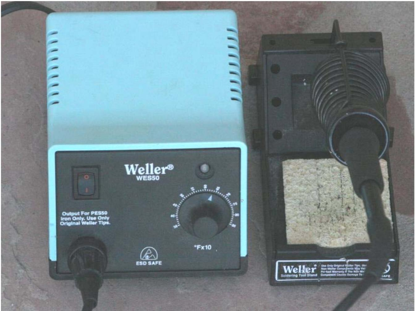
**Figure 2. A temperature controlled soldering helps a lot. 650 to 700 degrees is recommended.**
