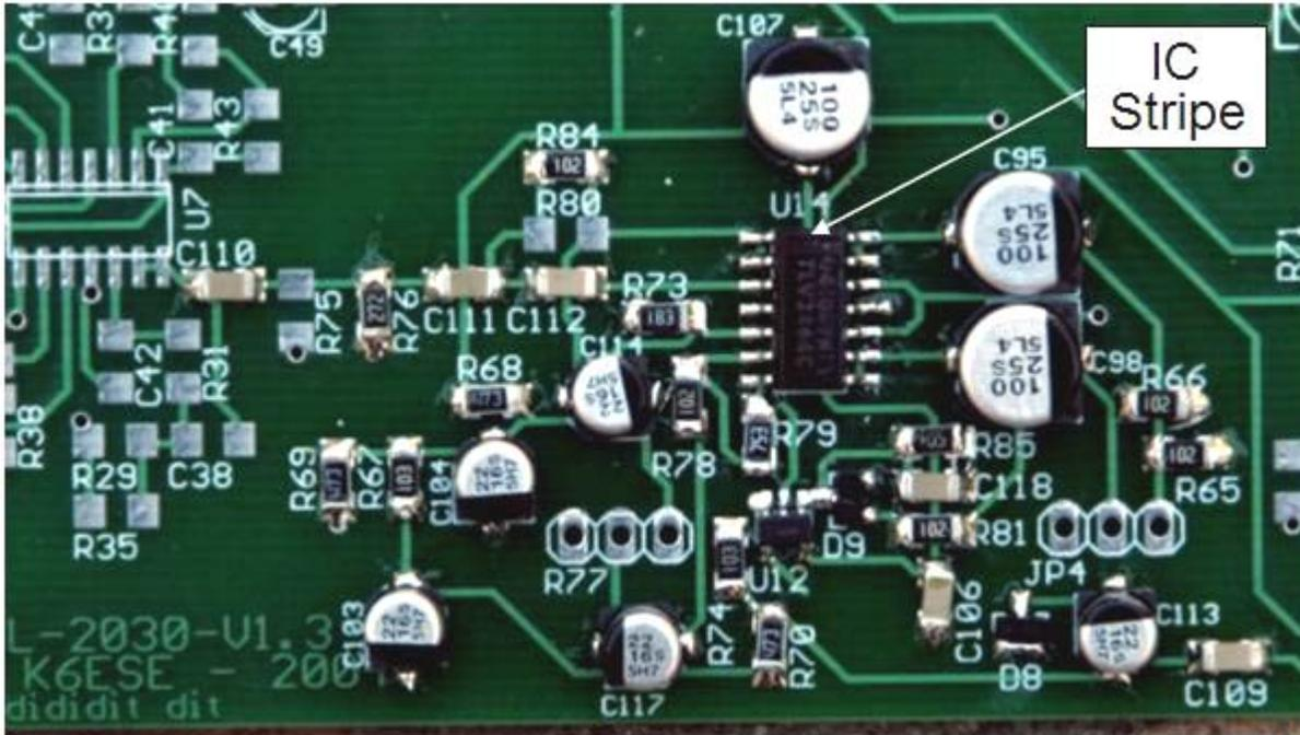
Figure 34. Picture shows orientation of U11 with stripe on upper end.
