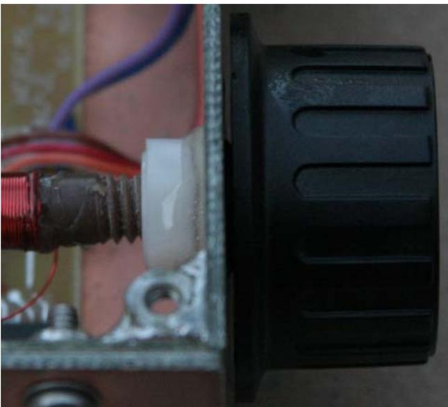
Figure 121. With PTO screw fully inserted, adjust tuning knob to have a small amount of front panel clearance.
