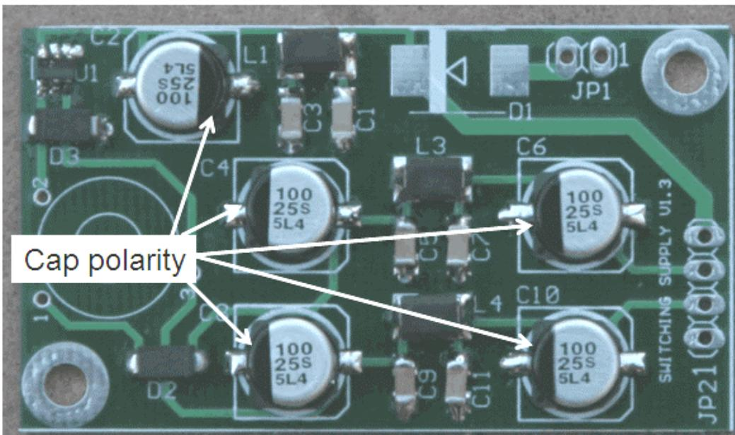
Figure 16. PS and Electrolytic Caps Polarity Details
