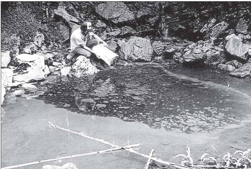
Plate 6.4. Andy Grubbs injecting dye in the San Andrés swallet.
