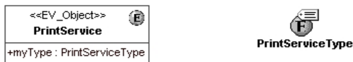
Figure 9 – An explicit representation of the type of an enterprise object so that the object can access its type
