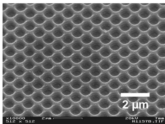
**Fig. 5** Two dimensional sub-μm pattern made by front side ablation in SiO<sub>x</sub> on fused silica, laser: 248 nm, 0.5 ps, 600 mJ/cm<sup>2</sup>, 7 pulses
