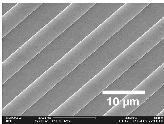
**Fig. 2** Pattern of 5  $\mu\text{m}$  lines and spaces made by rear side ablation in  $\text{SiO}_x$  on fused silica, laser: 193 nm, 20 ns, 540  $\text{mJ}/\text{cm}^2$ , 1 pulse
