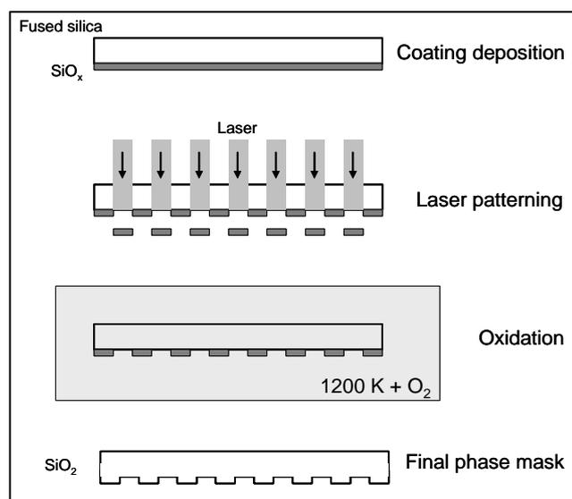
**Fig. 1** Process scheme for the laser based fabrication of  $\text{SiO}_2$  phase masks
