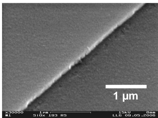
**Fig. 3** Ablation edge (detail of fig. 2), step height corresponds to the coating thickness of 250 nm
