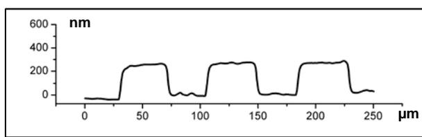
**Fig. 4** Surface profile of a SiO<sub>2</sub>-phase mask with 40 μm lines and spaces fabricated by the described method; Profile recorded with a Dektak stylus profilometer (note that the ordinate scale is in nm, the abscissa is in μm).
