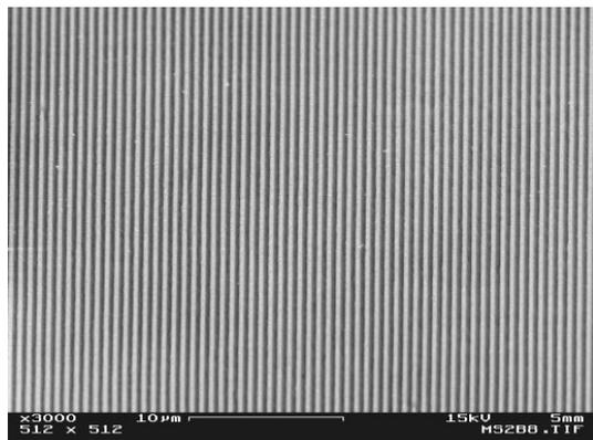
**Fig. 7** Sub- $\mu\text{m}$  line pattern ablated in steel, laser: 248 nm, 0.5 ps,  $500 \text{ mJ/cm}^2$ , 150 pulses
