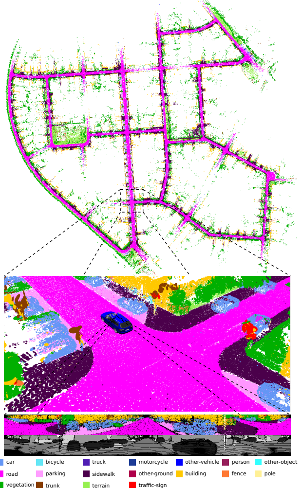
Fig. 1: Semantic map of the KITTI dataset generated with our approach using only LiDAR scans. The map is represented by surfels that have a class label indicated by the respective color. Overall, our semantic SLAM pipeline is able to provide high-quality semantic maps with higher metric accuracy than its non-semantic counterpart.
