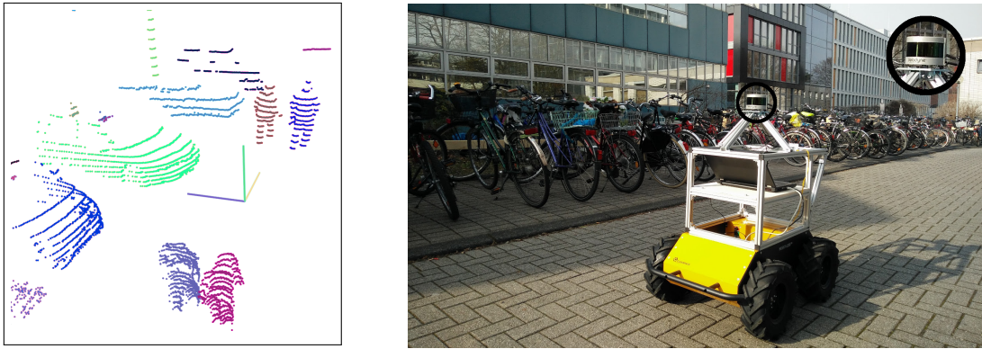
Figure 5.1: Left : Segmentation of objects such as people, cars, and trees generated from sparse 3D range data recorded with Velodyne VLP-16 scanner. Colors correspond to different segments. Right : Clearpath Husky robot used for the experiments driving at the University of Bonn campus.
