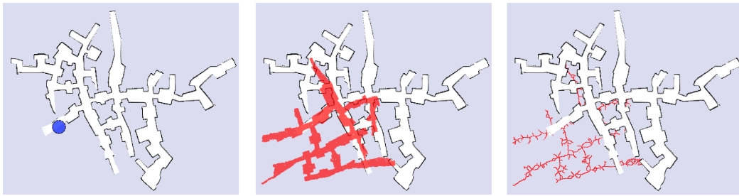
Figure 4.14: Illustration of the loop closures prediction. Left : So far explored map with the frontier under consideration (blue circle). Middle : One map from the predictive belief (in red) superimposed on the map explored so far. Right : Voronoi diagram used for the path search.
