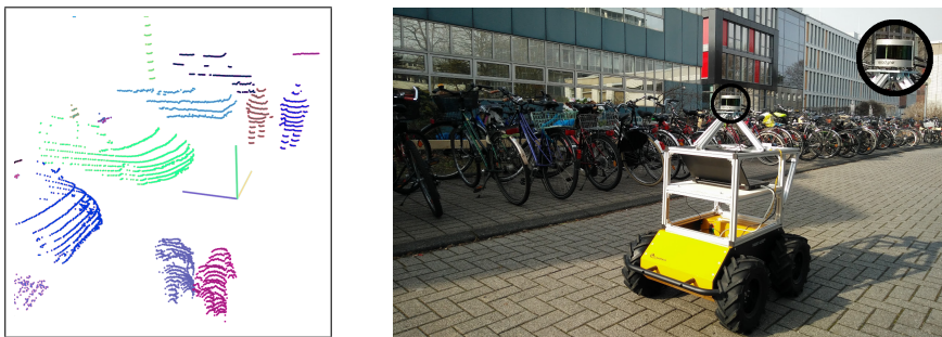
Fig. 1: Left: Segmentation of objects such as people, cars, and trees generated from sparse 3D range data recorded with Velodyne VLP-16 scanner. Colours correspond to different segments. Right: Clearpath Husky robot used for the experiments.
