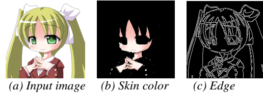
Fig. 2 Example of skin color and edge extraction, (a) an input image, (b) skin color extraction from (a), (c) edge extraction from (a).
