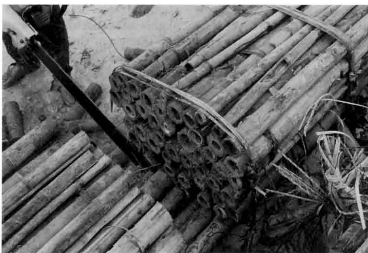
Figure 7. Destructive sampling of bamboo pontoon of Nale Tasih 1 with chainsaw. (Photo: author)
