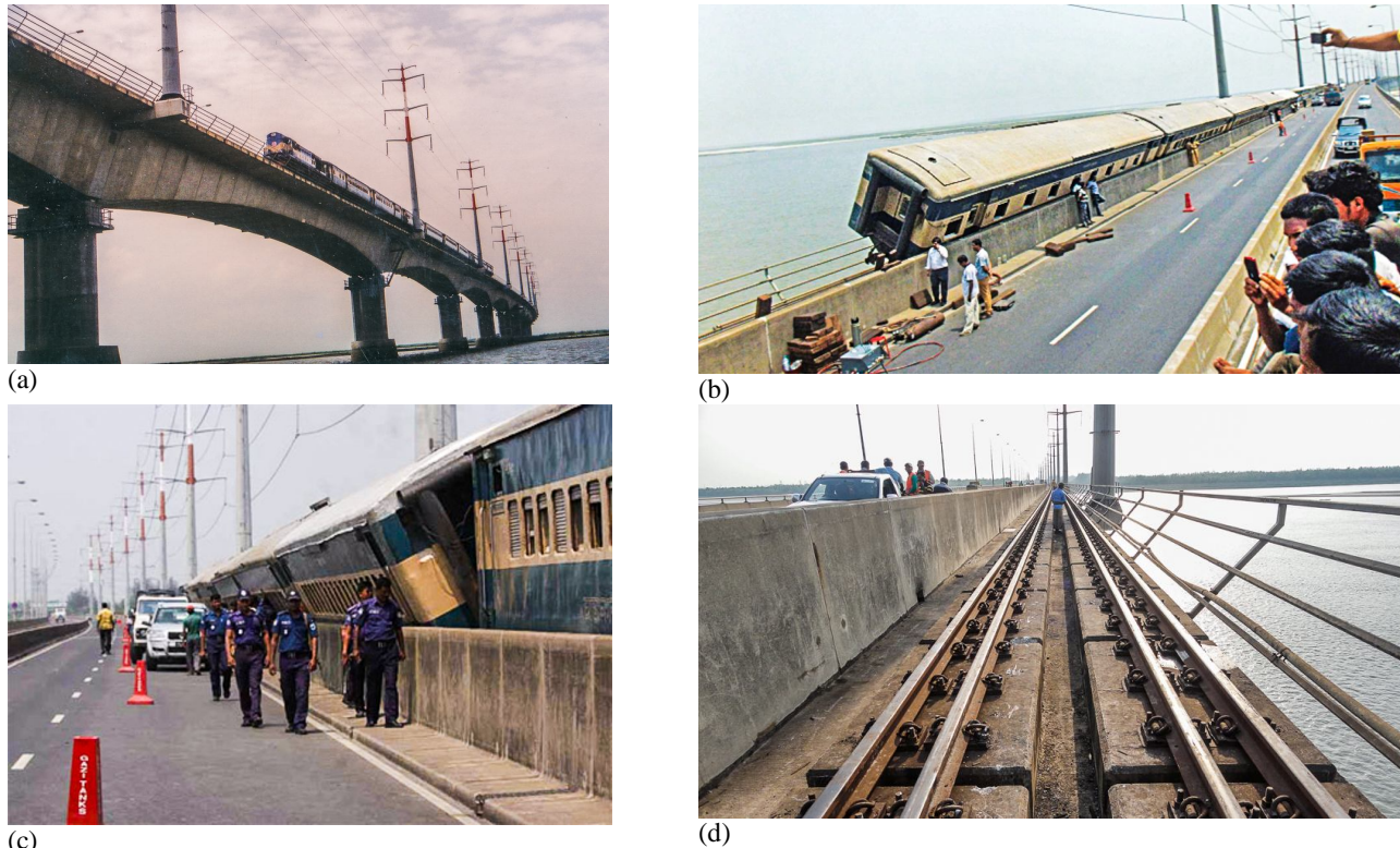
Figure 20. Over-turning of train at the Bangabandhu Jamuna Bridge. Source for (b)-(d): Press/news reports.
