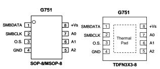
Note: Recommend connecting the Thermal Pad to the Ground or let it keep floating.
