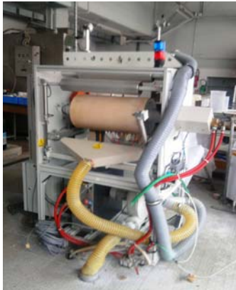
Fig.5. Utilajul COATING STAR - 1. Sample; 2. 2 Electrodes (1.5*50cm); 3.Roll shaped counted-electrode; 4. Aerosol inlet.
