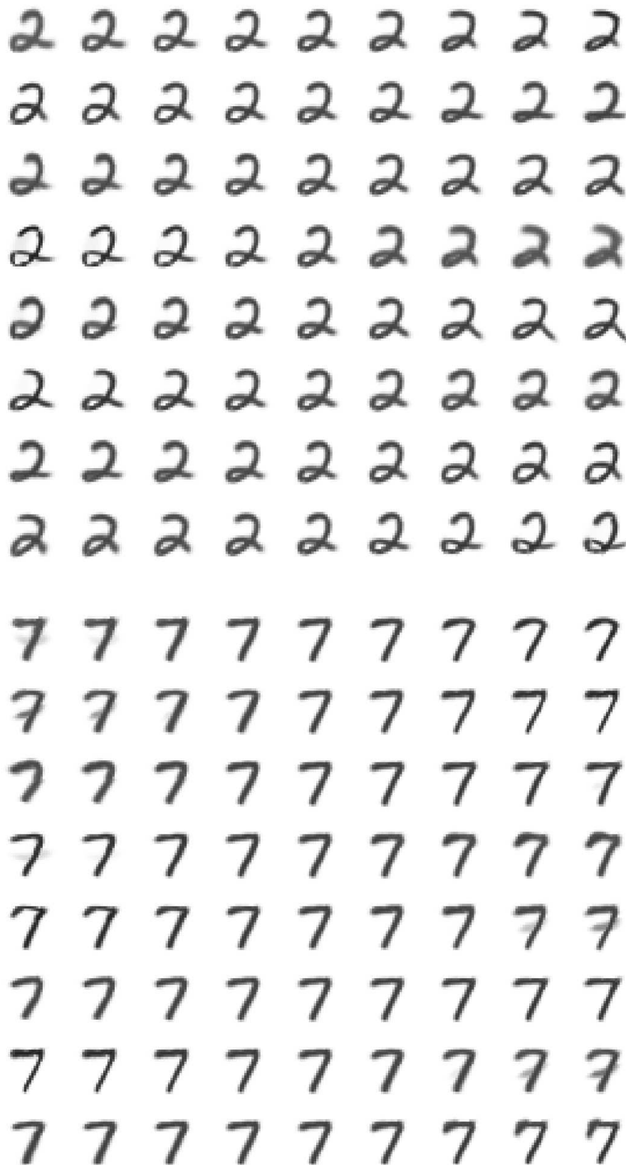
Figure 2.18: The effect of changing individual distortion variables, for two CCs. Notice how most distortion variables control only one or two aspects of the appearance: they're fairly specific. This is encouraged by applying dropout to the distortion variables (see Section 2.4.4).
