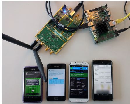
Figure 2: Our experimental setup with host and USRP. Phones are running the ICD apps.
