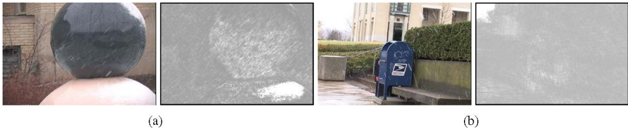
Fig. 10 One frame each from two sequences, and its corresponding correlation magnitude (Garg and Nayar 2004) (scaled linearly for display). (a) For the stationary sequence of the reflective ball, all of the current streaks are visible in the magnitude image, plus ghosts from
