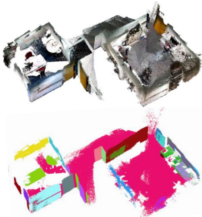
Fig. 6: Reconstruction of two rooms using our KDP-SLAM system (top) and its corresponding false-colored planar map (bottom).
