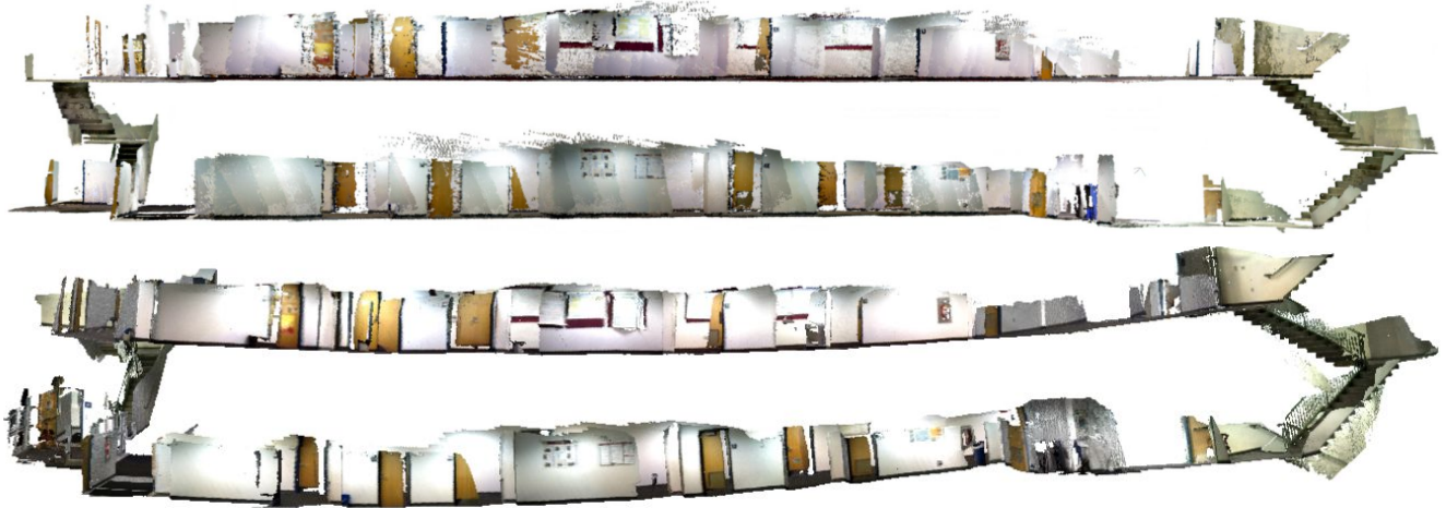
Fig. 7: Two floor dataset reconstructions by KDP-SLAM (top) and Kintinuous (bottom). Note that KDP-SLAM has reduced drift and maintained the planar structure after loop closure compared to Kintinuous.
