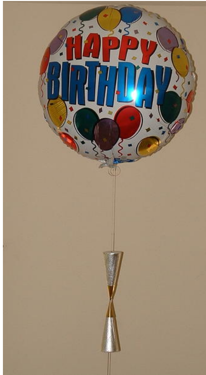
Illustration 14: "Featherweight" bi-conical antenna, integrated TM mode launcher and supporting balloon tethered by feed line.
