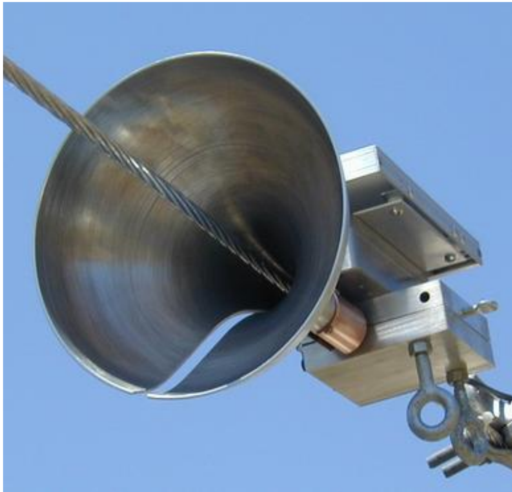
Illustration 9: A slotted E-Line launcher mounted to an aluminum power line conductor.
