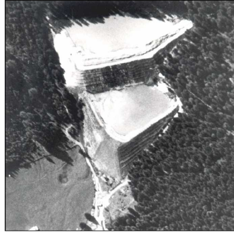
Fig. 6. The decantation basins photographed in September 1978 . The geometry of the upper basin seems altered with respect to the previous photo: works to raise the embankment according to the scheme “upstream” are clearly in progress (photo Impresa Rossi, Brescia).
