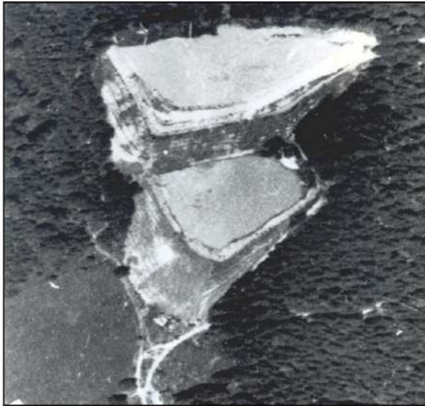
Fig. 7. The Pozzole basins in the summer 1983. The top of the upper embankment appears amply broadened and leveled. Also noticeable is the development of the delta deposit at the left end of the upper basin, next to the place of cyclone operation (photo Impresa Rossi, Brescia).
