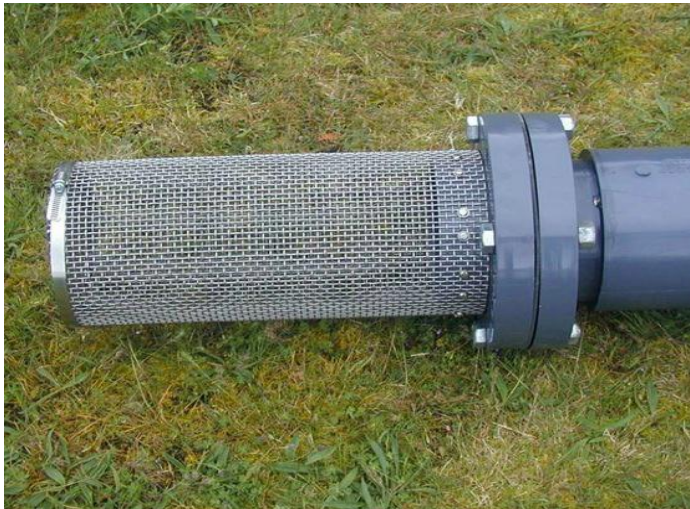
Fig 9 - Example of Diffuser
