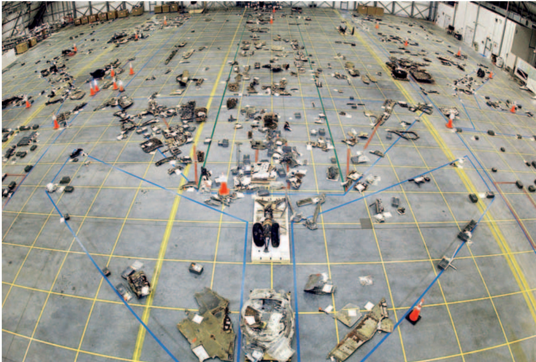
Hangar at Kennedy Space Center in Cape Canaveral, Florida, March 7, 2003, photo © NASA/Getty Images ■ NASA crash investigators place debris from the Space Shuttle Columbia onto a grid on the floor of a hangar. NASA is attempting to reassemble debris from the shuttle to learn what caused Columbia to break-up during reentry. NASA Mission Control lost contact with the Space Shuttle Columbia during the reentry phase of mission STS-107 on February 1, 2003 and later learned that the shuttle had broken up over Texas. Debris from the wreckage drifted hundreds of miles from central Texas to Louisiana. All seven astronauts onboard the shuttle died in the crash.
