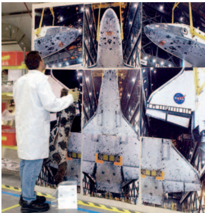
NASA Crash Investigator, Kennedy Space Center in Cape Canaveral, Florida, March 11, 2003, © photo: AP Photo/NASA, Kim Shiflett ■ A member of the space shuttle reconstruction project team holds a piece of wreckage and tries to locate it on pictures of Columbia taken while the orbiter was in the vehicle assembly building.
