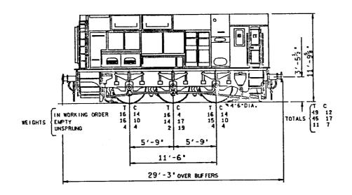
350 H.P.B.R.O-6-0 DIESEL ELECTRIC SHUNTING LOCOMOTIVE
