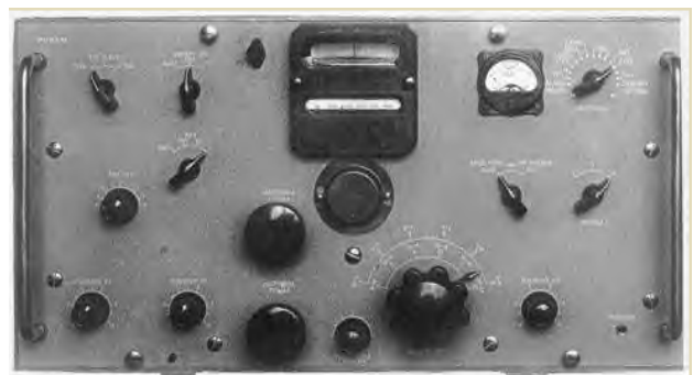
Communications receivers "Krot-M" (USSR), used for tracking of the jamming targets in the 50's and 60's.
