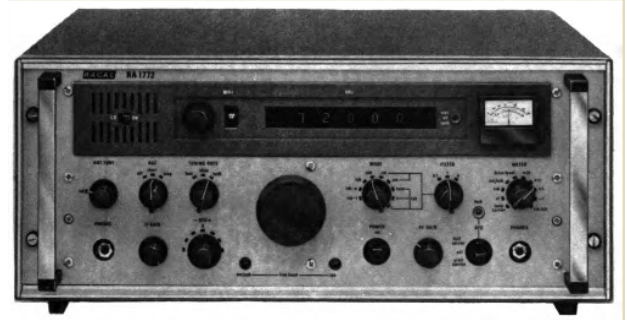
Racal "RA-1772" (UK) communications receivers, used for tracking of the jamming targets in the 70's and 80's at the receiving station near Warsaw.
