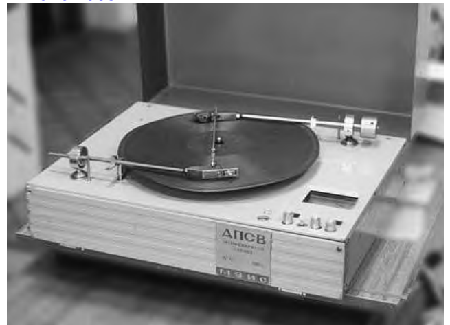
Device for playback of the "speech-like" jamming audio signal
