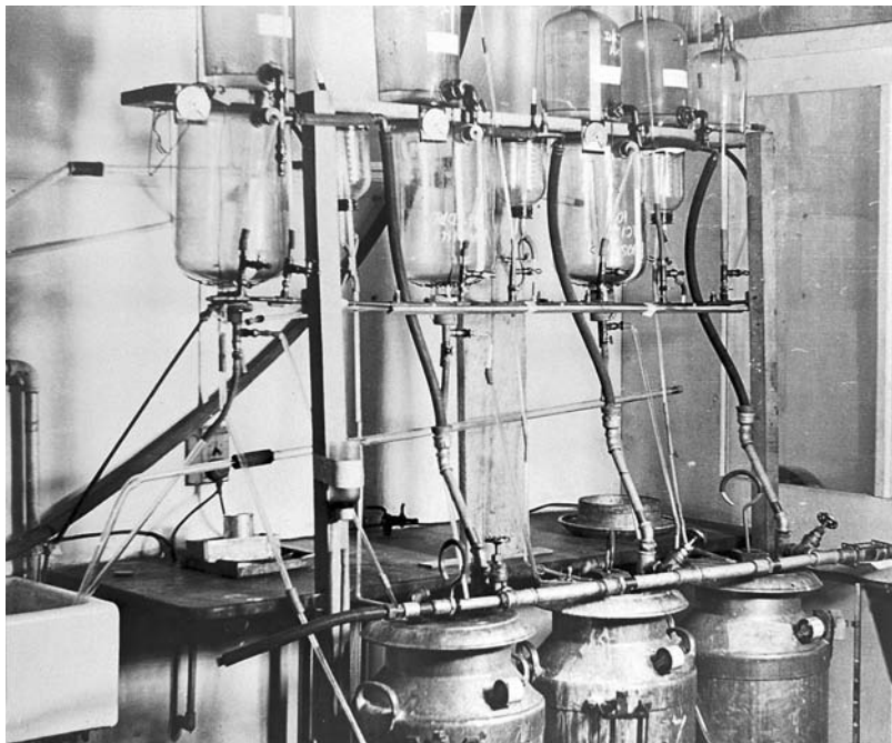
Equipment used for making early forms of penicillin; glass flasks and leads into tops of milk-churns. Wellcome Library, London.
