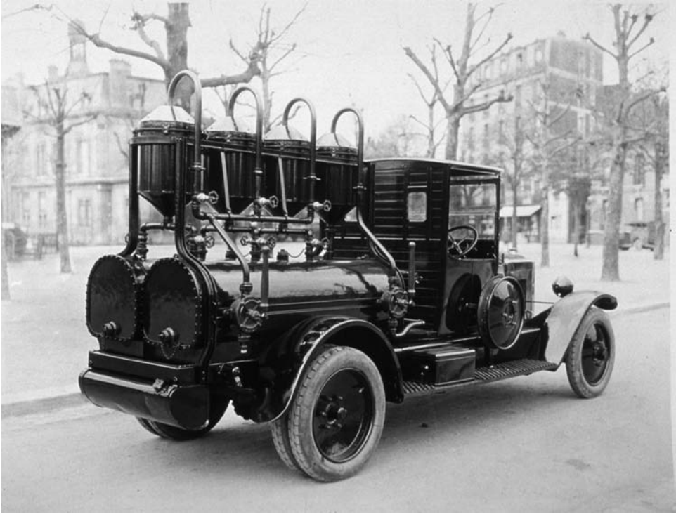
Truck equipped with disinfection tanks. Courtesy of the National Library of Medicine.
