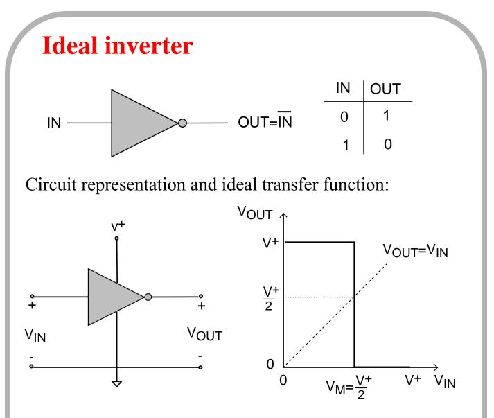
Define *switching point* or *logic threshold* :
