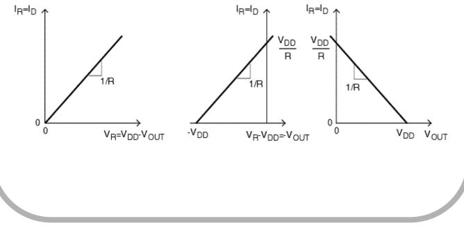
Overlap I–V characteristics of resistor pull-up on I–V characteristics of transistor:
