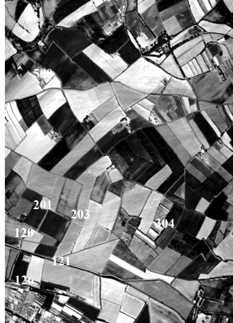
Figure 36. Image of radiance at the sensor (no atmospheric correction) for DAIS channel 76, showing part of the ReSeDA test site with some selected plots indicated. North is up. Radiances range approximately from 0.92 to 1.51 \text{ mW/cm}^2 \text{ sr } \mu\text{m} ( 23 to 58 \text{ }^\circ\text{C} ).
