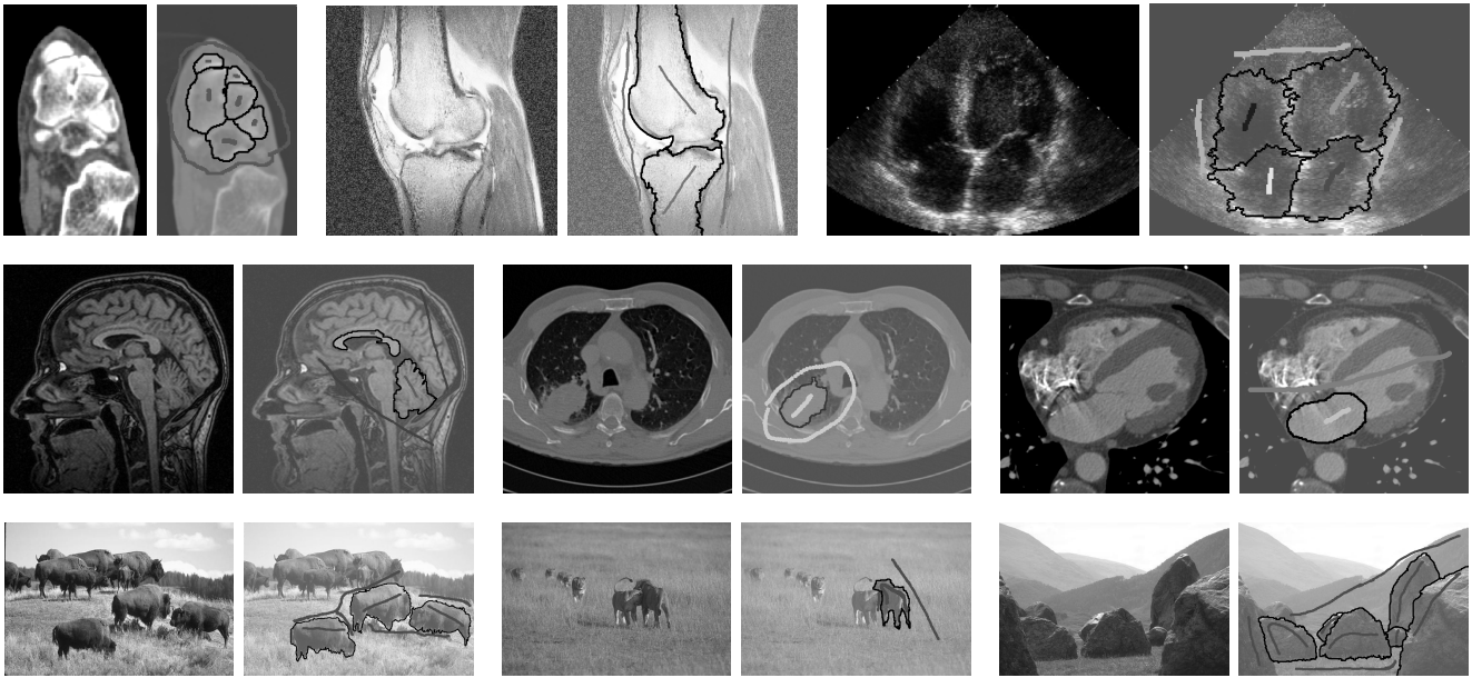
Fig. 8. Examples of segmentations on medical and non-medical images. We stress that the edge weights are based upon intensity differences alone, although more advanced intensity/texture analysis could be used in a particular problem domain. The thick, gray lines (chosen to maximize contrast) represent the seed points and the thick black lines represent the segment boundaries. Note that the processed images were whitened in order to accentuate the seeds and the segmentation boundary. The same parameter value ( \beta = 900 ) and 4-connected lattice topology were used for all segmentations.
