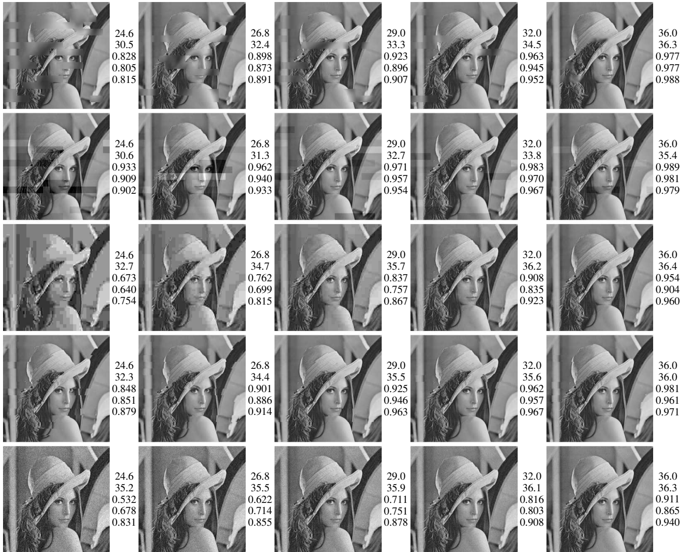
Fig. 7. Example realistic distortion images where columns have approximately equal PSNR. From top to bottom row, the distortions are (1) block blur, (2) block intensity shift, (3) JPEG compression, (4) block spatial shift, and (5) additive white noise. The metric values to the right of the images correspond to PSNR, Perceptual PSNR, SSIM, CWSSIM, and WCWSSIM.
