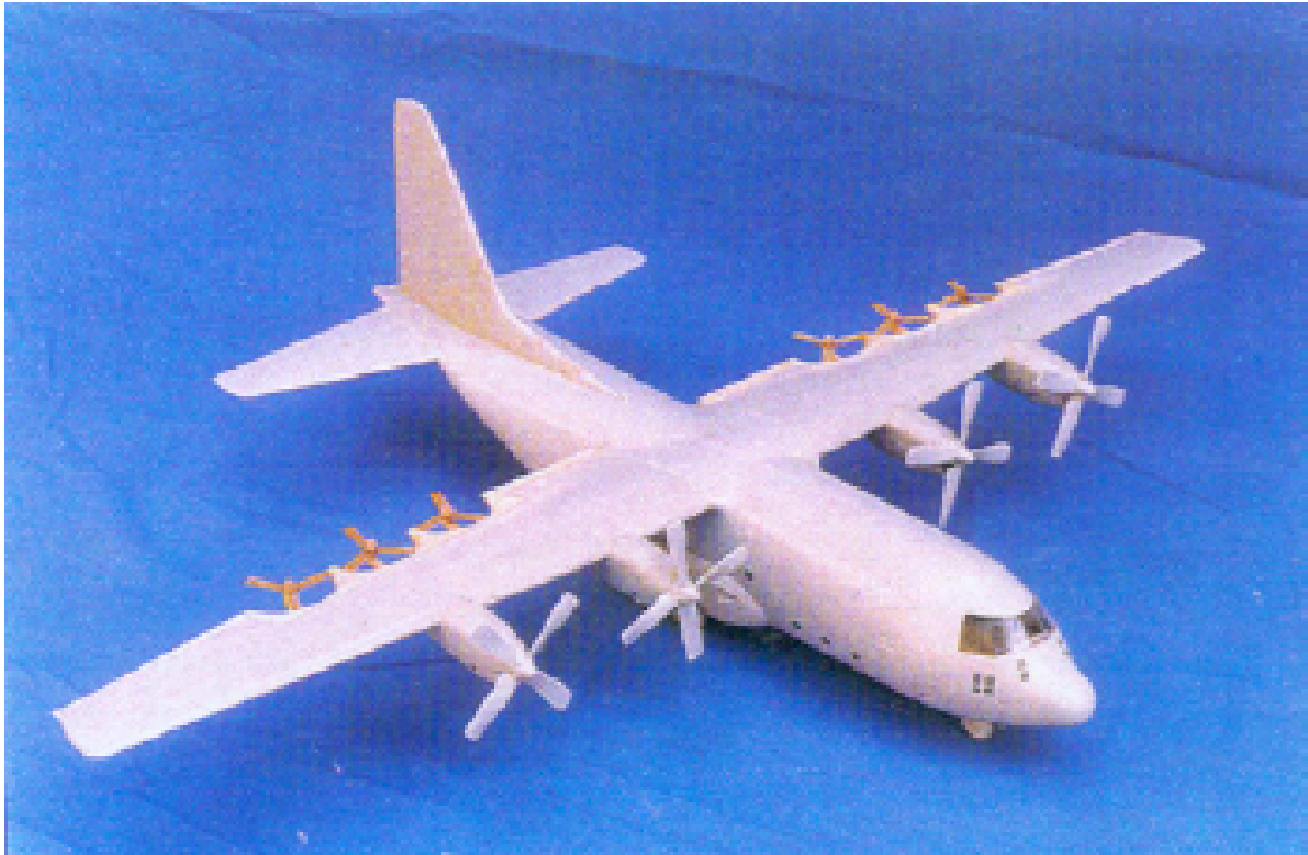
Model of a Lockheed C-130 equipped with Turbo Wings Showing the flaps removed and rotors installed
