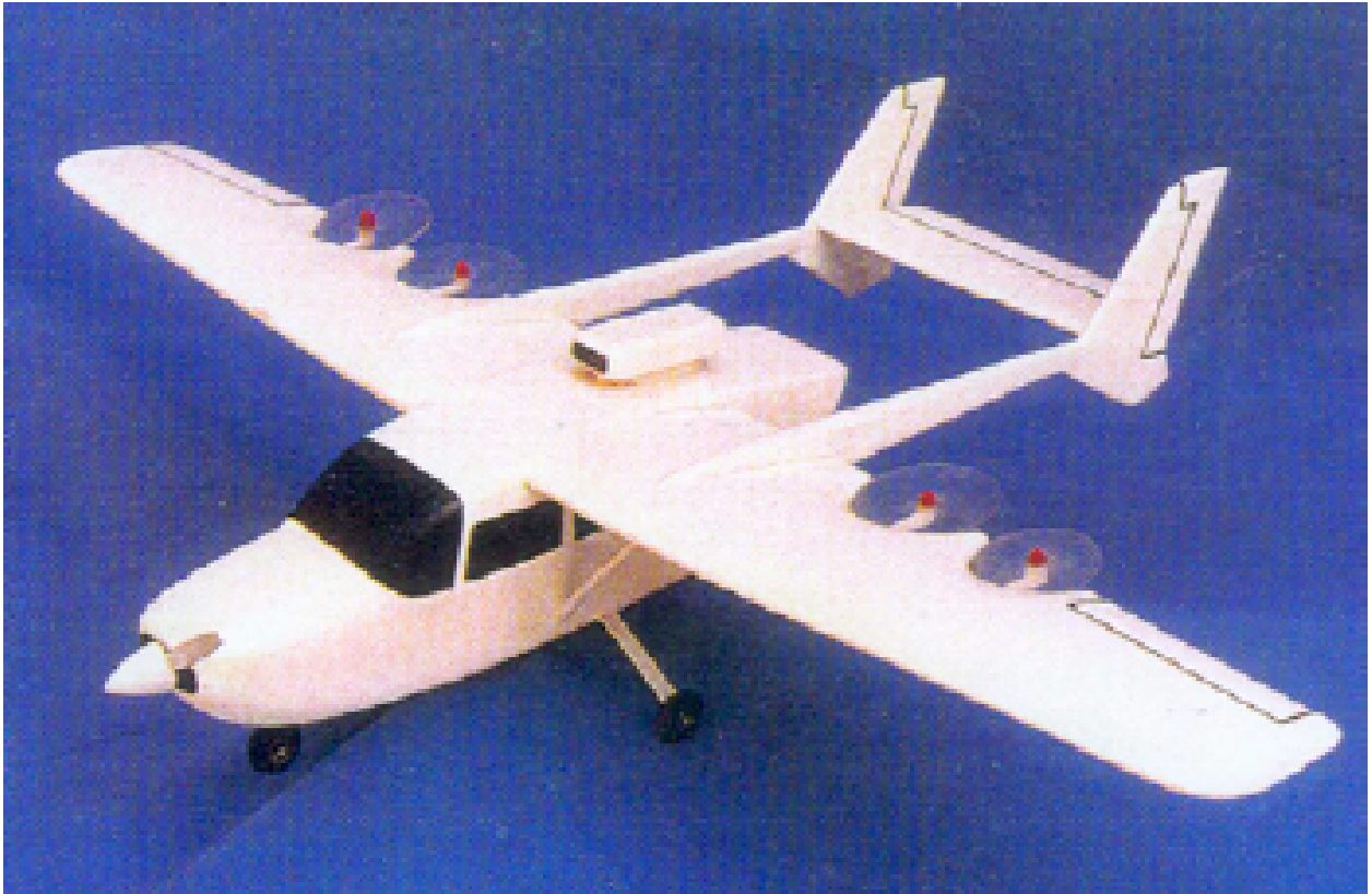
Model of a Cessna 337 equipped with Turbo Wings Showing the flaps removed and rotors installed
