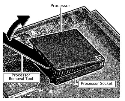
Position the teeth of the processor removal tool in the groove between the processor and the logic board socket.
