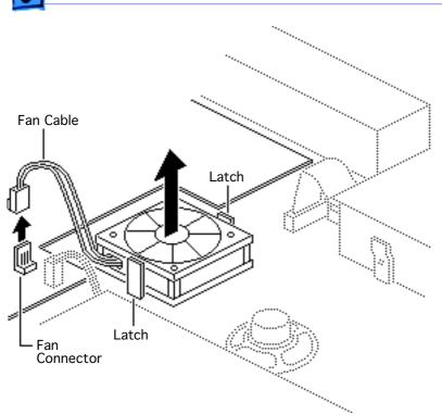
Disconnect the fan cable from the fan connector on the logic board.
