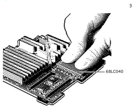
Caution: Forcing the 68LC040 processor connector pins into the socket could damage the pins. If the processor resists installation, check the pin alignment.
