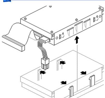
Release the two plastic latches on one side of the hard drive and lift the drive slightly. Repeat on the other side of the drive and remove the drive (with carrier) from the computer.
