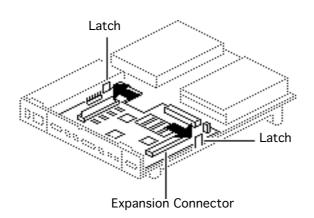
3 **Caution:** Using your forefingers, spread the two latches that secure the logic board to the bottom case. At the same time, using your right thumb, push on the expansion connector and slide the logic board toward the front of the case.
