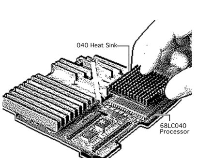
6 Peel the paper from the back of the heat sink and install the heat sink on the processor.
