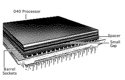
**Note:** On a correctly installed 040 processor, a very small gap separates the 040 chip from the metal spacer. A larger gap caused by the board barrel sockets separates the upgrade board and the spacer.
