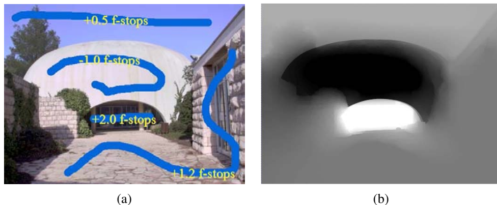
Figure 10.28 Interactive local tone mapping (Lischinski, Farbman, Uyttendaele et al. 2006b) © 2006 ACM: (a) user-drawn strokes with associated exposure values g(x, y) (b) corresponding piecewise-smooth exposure adjustment map f(x, y) .
