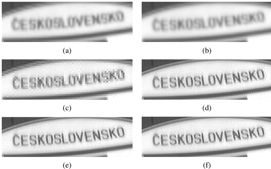
Figure 10.31 Super-resolution results using a variety of image priors (Capel 2001): (a) Low-res ROI (bicubic 3\times zoom); (b) average image; (c) MLE @ 1.25\times pixel-zoom; (d) simple \|x\|^2 prior ( \lambda = 0.004 ); (e) GMRF ( \lambda = 0.003 ); (f) HMRF ( \lambda = 0.01, \alpha = 0.04 ). 10 images are used as input and a 3\times super-resolved image is produced in each case, except for the MLE result in (c).
