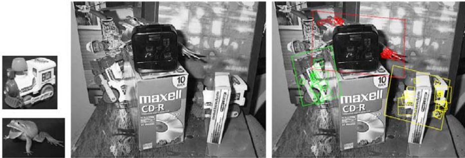
Figure 4.21 Recognizing objects in a cluttered scene (Lowe 2004) © 2004 Springer. Two of the training images in the database are shown on the left. These are matched to the cluttered scene in the middle using SIFT features, shown as small squares in the right image. The affine warp of each recognized database image onto the scene is shown as a larger parallelogram in the right image.
