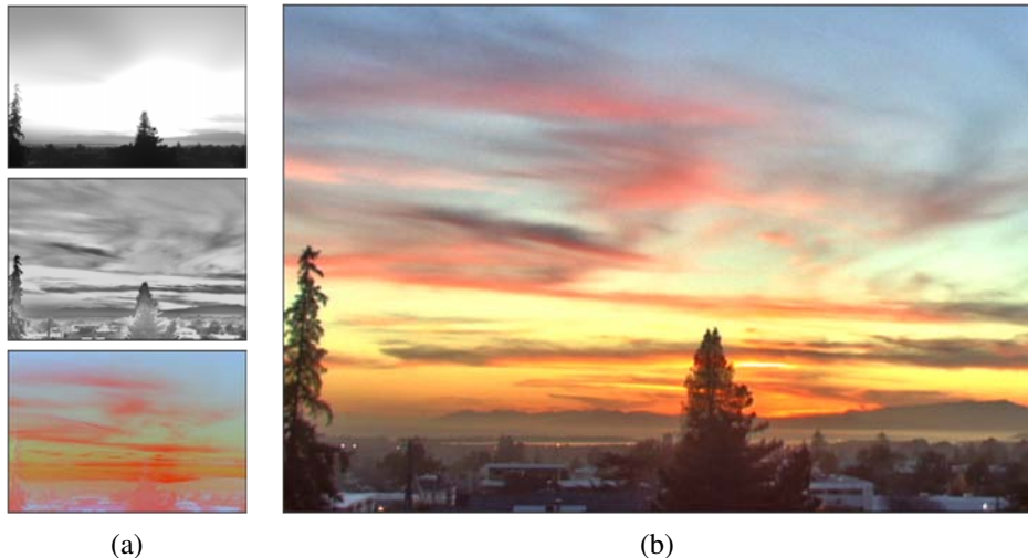
Figure 10.22 Local tone mapping using bilateral filter (Durand and Dorsey 2002): (a) low-pass and high-pass bilateral filtered log luminance images and color (chrominance) image; (b) resulting tone-mapped image (after attenuating the low-pass log luminance image) shows no halos. Processed images courtesy of Frédo Durand, MIT 6.815/6.865 course on Computational Photography.
