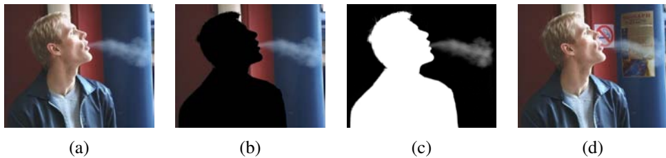
Figure 10.47 Smoke matting (Chuang, Agarwala, Curless et al. 2002) © 2002 ACM: (a) input video frame; (b) after removing the foreground object; (c) estimated alpha matte; (d) insertion of new objects into the background.
