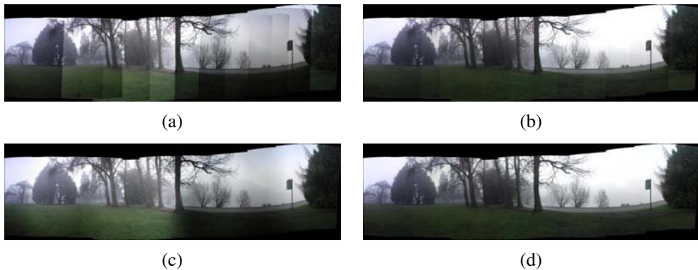
Figure 10.6 Simultaneous estimation of vignetting, exposure, and radiometric response (Goldman 2011) © 2011 IEEE: (a) original average of the input images; (b) after compensating for vignetting; (c) using gradient domain blending only (note the remaining mottled look); (d) after both vignetting compensation and blending.
