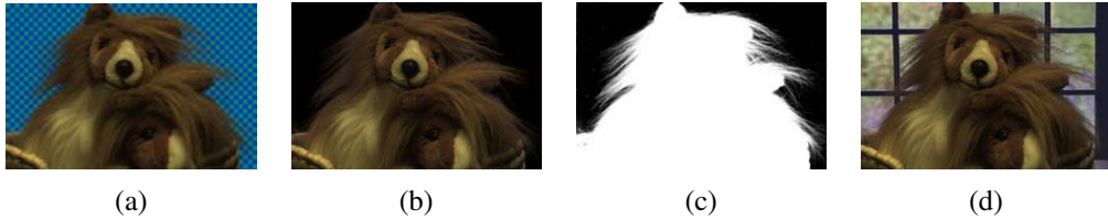
Figure 3.4 Image matting and compositing (Chuang, Curless, Salesin et al. 2001) © 2001 IEEE: (a) source image; (b) extracted foreground object F ; (c) alpha matte \alpha shown in grayscale; (d) new composite C .
