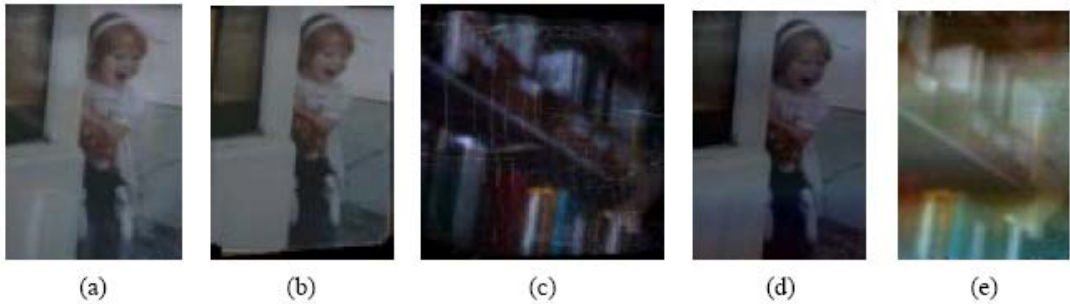
Figure 8.18 Transparent motion separation (Szeliski, Avidan, and Anandan 2000) © 2000 IEEE: (a) first image from input sequence; (b) dominant motion layer min-composite ; (c) secondary motion residual layer max-composite ; (d–e) final estimated picture and reflection layers. Note that the reflected layers in (c) and (e) are doubled in intensity to better show their structure.
