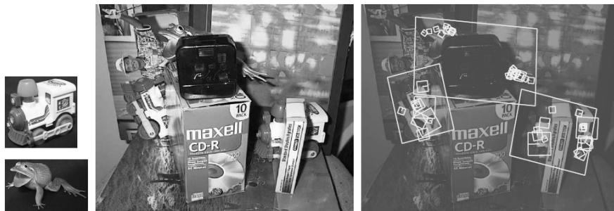
Figure 14.26 Recognizing objects in a cluttered scene (Lowe 2004) © 2004 Springer. Two of the training images in the database are shown on the left. They are matched to the cluttered scene in the middle using SIFT features, shown as small squares in the right image. The affine warp of each recognized database image onto the scene is shown as a larger parallelogram in the right image.
