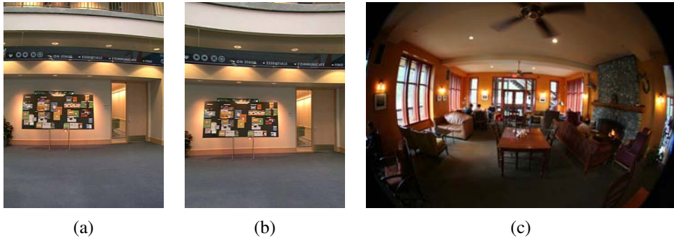
Figure 2.13 Radial lens distortions: (a) barrel, (b) pincushion, and (c) fisheye. The fisheye image spans almost 180^\circ from side-to-side.
