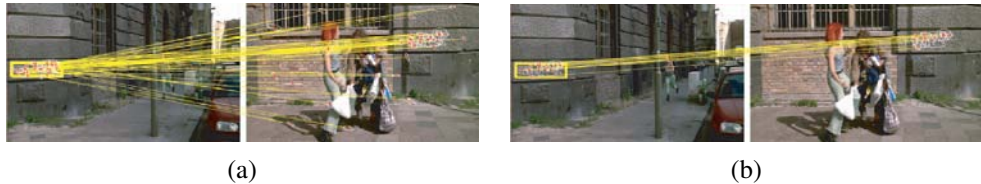
Figure 14.29 Matching based on visual words (Sivic and Zisserman 2009) © 2009 IEEE. (a) Features in the query region on the left are matched to corresponding features in a highly ranked video frame. (b) Results after removing the stop words and filtering the results using spatial consistency.
