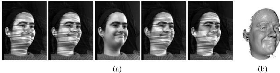
Figure 12.7 Real-time dense 3D face capture using spacetime stereo (Zhang, Snavely, Curless et al. 2004) © 2004 ACM: (a) set of five consecutive video frames from one of two stereo cameras (every fifth frame is free of stripe patterns, in order to extract texture); (b) resulting high-quality 3D surface model (depth map visualized as a shaded rendering).
