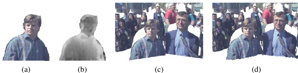
Figure 13.6 Sprites with depth (Shade, Gortler, He et al. 1998) © 1998 ACM: (a) alpha-matted color sprite; (b) corresponding relative depth or parallax; (c) rendering without relative depth; (d) rendering with depth (note the curved object boundaries).
