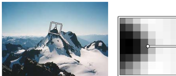
Figure 4.17 MOPS descriptors are formed using an 8 \times 8 sampling of bias and gain normalized intensity values, with a sample spacing of five pixels relative to the detection scale (Brown, Szeliski, and Winder 2005) © 2005 IEEE. This low frequency sampling gives the features some robustness to interest point location error and is achieved by sampling at a higher pyramid level than the detection scale.
