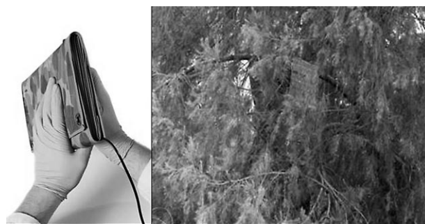
Figure 20. The flexible DSSC-based solar module developed by Dyesol for the Australian Army camouflages itself in trees where it provides constant voltage under a wide range of illumination levels (photo courtesy of Dyesol).
