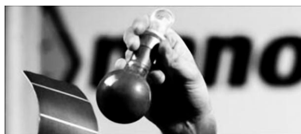
Figure 4. Nano ink: The ink serves a useful purpose by effectively locking in a uniform distribution. The homogeneous mixture of nanoparticles in the ink in suitable overall amounts ensures that the atomic ratios of the four elements (copper, indium, gallium, selenium) are correct even across large areas of deposition (photo courtesy of Nanosolar).
