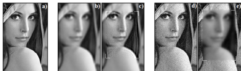
Figure: (a) Original image, (b) Blurred and slightly noisy image, (c) Restored version of (b), (d) No blur, severe noise, (e) Restored version of (d).
