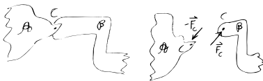
Figure 10.24: A frictionless hinge is a workless constraint. The net work of the interaction force on the two contacting bodies is zero.
