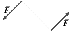
Figure 2.54: One couple. The forces add to zero. Then net moment they cause does not.
