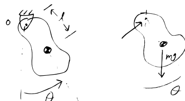
Figure 10.26: A rigid body suspended from a frictionless hinge is an energy conserving one-degree-of-freedom mechanism.
