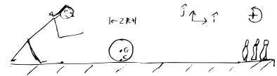
Figure 8.32: The bowling ball is sliding so long as v_G \neq -\omega R
