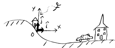
Figure 9.18: A fixed reference frame \mathcal{F} is defined by an origin 0 and coordinate axes xyz or base vectors \hat{i}\hat{j}\hat{k} . Once the xy (or \hat{i}\hat{j} ) directions are chosen the z (or \hat{k} ) direction is implicitly defined by the right hand rule.
