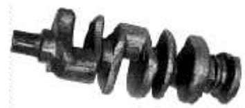
Figure 11.1: A car crankshaft is a complex three-dimensional object which is well approximated for many purposes as rotating about a fixed axis. The relative timing of the reciprocating pistons is controlled by this complex shape. “Connecting rods” are pinned to the cylinders at one end and to the short offset cylinders on the crankshaft at the other.
