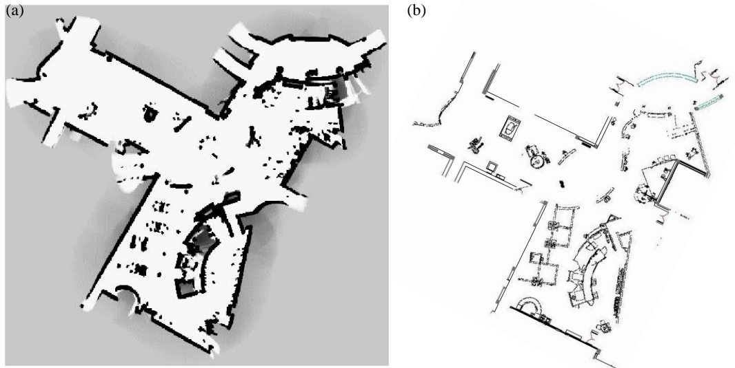
Figure 9: (a) Occupancy grid map and (b) architectural blueprint of a recently constructed building. The blueprint is less accurate than the map in several locations.
