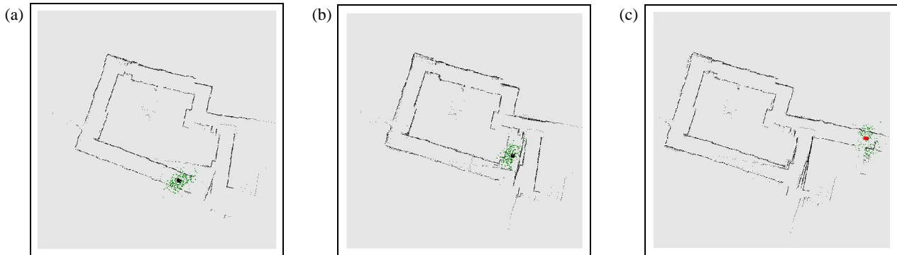
Figure 7: Hybrid approach, which maintains a posterior estimate over the robot poses, represented by a set of particles. When closing the loop, these samples are used to relocalize the robot in the map and correct the map accordingly.
